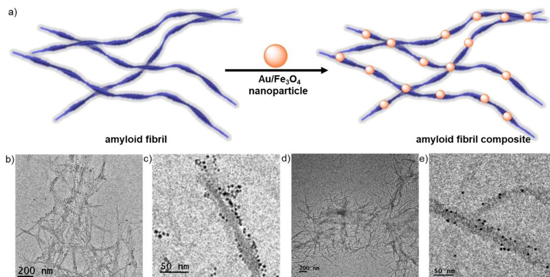
Fig. 1 (a) Schematic representation of amyloid fibrils and their gold/iron oxide composites. TEM images of amyloid–Au (b and c) and amyloid–Fe<sub>3</sub>O<sub>4</sub> (d and e) composites. The magnified images demonstrate the attachment of Au/Fe<sub>3</sub>O<sub>4</sub> nanoparticles with amyloid fibrils.
