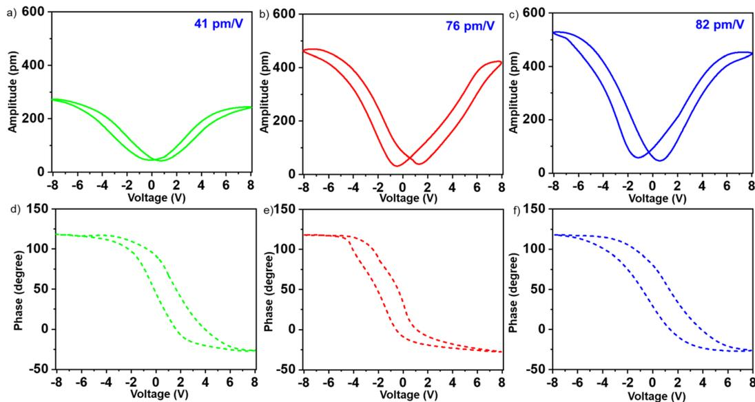
Fig. 2 Amplitude-voltage butterfly loops of amyloid fibril (a), amyloid-Au (b) and amyloid-Fe<sub>3</sub>O<sub>4</sub> (c) with piezoelectric constant values shown as insets. Phase hysteresis loops of amyloid fibril (d), amyloid-Au (e) and amyloid-Fe<sub>3</sub>O<sub>4</sub> (f).
