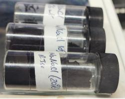
Fig. 2 Free-flowing black powders of 5, 10, 20% w/w Na/NaCl, respectively, made via planetary ball-milling
