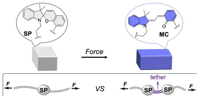
Fig. 1 Spiropyran-based mechanochemical polymer materials, and amplification of spiropyran activation in bulk materials through a tethering strategy.
