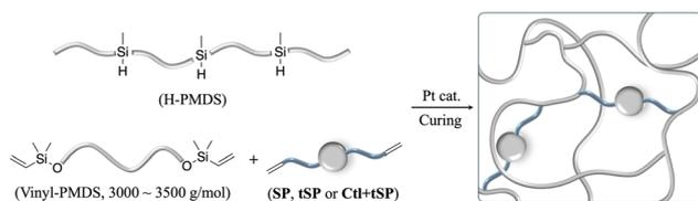
**Fig. 2** Schematic incorporation of a mechanophore linker into PDMS elastomer networks using the commercial Sylgard 184 kit. The amount of added SP, tSP or Ctl+tSP diene is less than 2.2 mol% or 4.4 mol% relative to vinyl-PDMS.
