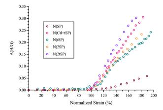
Fig. 4 Overlay of the representative set of  $\Delta(B/G)$  values for the samples under study. The strain was normalized to the activation onset strain.
