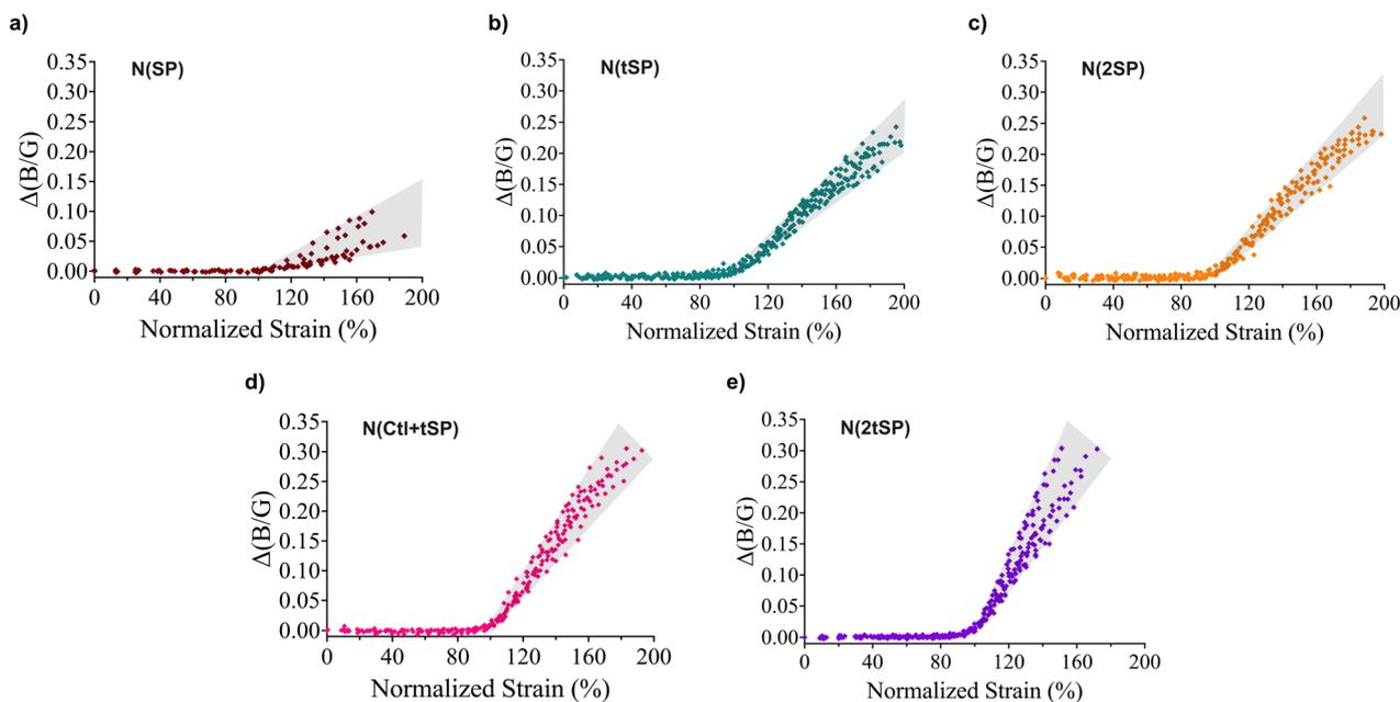
Fig. 5 Compiled plot of  $\Delta(B/G)$  against normalized strain for all samples. (a) **N(SP)**, (b) **N(tSP)**, (c) **N(2SP)**, (d) **N(Ctl+tSP)**, and (e) **N(2tSP)**. The strain was normalized to the activation onset, and the range of slope values is indicated by the grey area.
