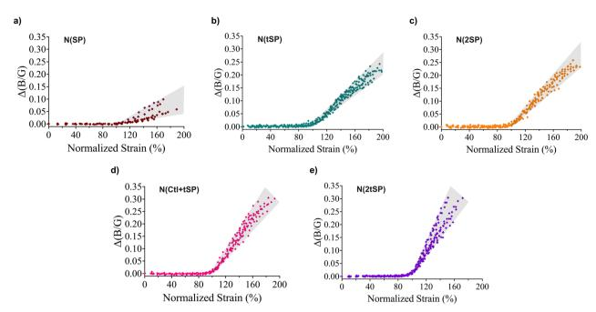
Fig. 5 Compiled plot of  $\Delta(B/G)$  against normalized strain for all samples. (a) N(SP), (b) N(tSP), (c) N(2SP), (d) N(Ctl+tSP), and (e) N(2tSP). The strain was normalized to the activation onset, and the range of slope values is indicated by the grey area.
