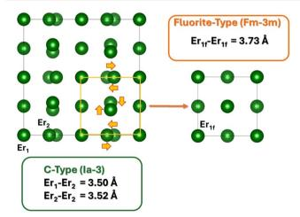
Fig. 8 Rational prospect of the structural changes of C-Er<sub>2</sub>O<sub>3</sub> taking place during high frequency ball milling. The oxygen positions are neglected for clarity, whereas the green spheres represent the Er<sup>3+</sup> crystal sites. The orange arrows define the atomic rearrangement of Er<sup>3+</sup> occurring during the structural conversion into fluorite-type. The average Er-Er interatomic distances are reported for both phases, as determined by structural refinements
