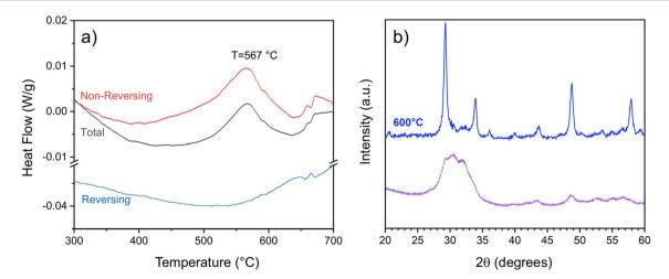
Fig. 5 (a) MDSC analysis performed on the  $B-Er_2O_3$  phase stabilized at 30 Hz for 6 h (exothermic event is shown upward). (b) PXRD measurements before and after annealing at 600 °C for 1 h.
