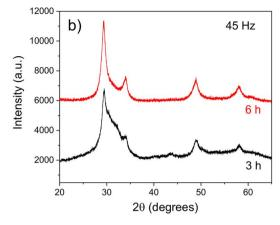
(a) PXRD data for Er<sub>2</sub>O<sub>3</sub> subjected to 40 Hz for 3 and 6 h. (b) PXRD data for Er<sub>2</sub>O<sub>3</sub> subjected to 45 Hz for 3 and 6 h.
