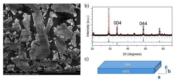
Fig. 1 (a) SEM micrograph showing the elongated platelet-like shape of Er<sub>2</sub>O<sub>3</sub> crystals prior to milling. (b) Direct comparison of the calculated (red line) and experimental (black symbols) diffraction patterns. The preferred orientation of the microcrystals is evidenced by the observed intensity of the 044 reflection. (c) Proposed crystal habit indicating the extension of the 0hh faces, in agreement with SEM and XRD measurements.
