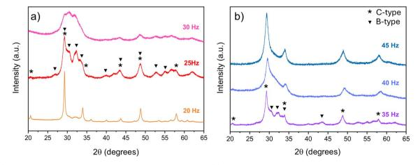
Fig. 2 (a) PXRD for  $Er_2O_3$  milled at frequencies from 20 to 30 Hz for 6 h. (b) PXRD for  $Er_2O_3$  milled at frequencies ranging from 35 Hz to 45 Hz for 6 h.
