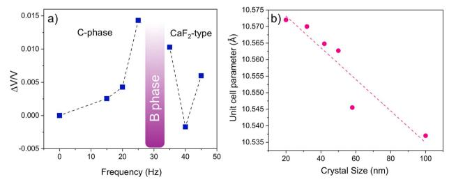
Fig. 4 (a) Volume changes ( $\Delta V/V$ ) for the C-polymorph and fluorite-type phase (using 2  $\times$   $V_{fluorite}$  for direct comparison) across all milling frequencies (15–45 Hz) after 6 hours processing. The unit cell parameters were determined by Rietveld refinements. (b) Dependence of the unit cell parameter on the crystal size for the C-polymorph determined by W-H method. The dotted line represents the linear regression.
