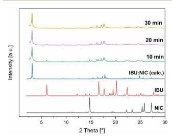
Fig. 3 PXRD pattern of NIC (black), IBU (red), calculated IBU:NIC cocrystal (blue), and of the reaction mixture after 10 min (green), 20 min (purple), 30 min (yellow) of milling at 500 rpm in attritor mill.
