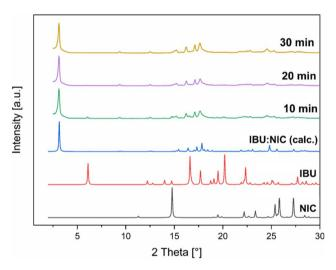
Fig. 5 PXRD pattern of NIC (black), IBU (red), calculated IBU:NIC cocrystal (blue), and of the reaction mixture after 10 min (green), 20 min (purple), 30 min (yellow) of milling at 800 rpm in attritor mill.
