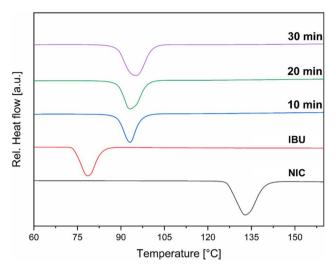
Fig. 4 DSC thermogram, showing NIC (black, m.p.: 130-132 °C), IBU (red, m.p.: 75-77 °C), and the reaction mixture after 10 min (blue), 20 min (green), and 30 min (purple) of milling at 800 rpm in attritor mill (IBU:NIC co-crystal, m.p.: 90-92 °C).
