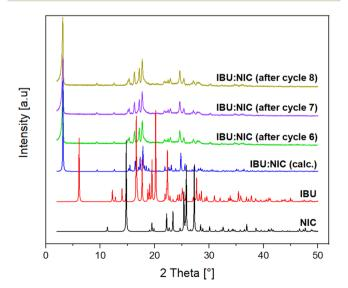
Fig. 6 PXRD pattern of NIC (black), IBU (red), calculated IBU:NIC cocrystal (blue), and of the reaction mixture after 6 cycles (green), 7 cycles (purple), 8 cycles (yellow) of sequential batch processing milling at 800 rpm in attritor mill.
