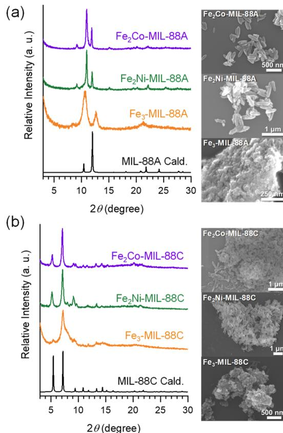
Fig. 3 (a) PXRD patterns and SEM images of  $Fe_2Co$ -MIL-88A,  $Fe_2Ni$ -MIL-88A, and  $Fe_3$ -MIL-88A after drying. (b) PXRD patterns and SEM images of  $Fe_2Co$ -MIL-88C,  $Fe_2Ni$ -MIL-88C, and  $Fe_3$ -MIL-88C after drying.
