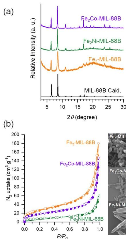
**Fig. 2** (a) PXRD patterns of  $\text{Fe}_3$ -MIL-88B,  $\text{Fe}_2\text{Co}$ -MIL-88B, and  $\text{Fe}_2\text{Ni}$ -MIL-88B collected after isolation from DMF. (b)  $\text{N}_2$  isotherms at  $77\text{ K}$  and SEM images of  $\text{Fe}_3$ -MIL-88B,  $\text{Fe}_2\text{Co}$ -MIL-88B, and  $\text{Fe}_2\text{Ni}$ -MIL-88B.
