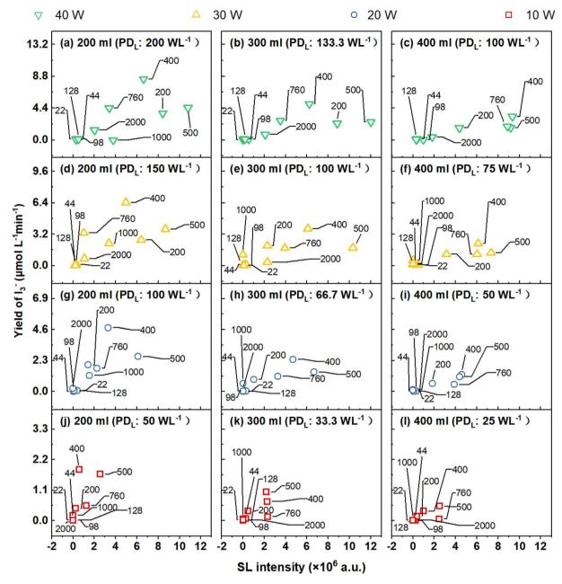
Fig. 17 The correlation between I<sub>3</sub><sup>-</sup> and SL generated during sonication (testing frequencies are labelled (kHz)): (a–c) 40 W, (d–f) 30 W, (g–i) 20 W and (j-l) 10 W.
