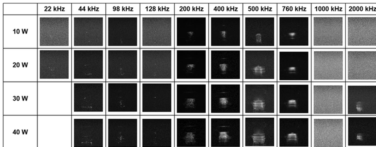
Fig. 4 Sono-/sonochemi-luminescence intensity distribution for all testing frequencies and powers at 300 ml reactor volume: (a) SL and (b) SCL.
