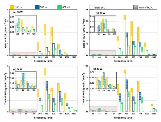
Fig. 12 The dosimetry results for quantification of IORS, H<sub>2</sub>O<sub>2</sub> and total ROS with different frequencies and solution volume: (a) 10 W, (b) 20 W, (c) 30 W and (d) 40 W.
