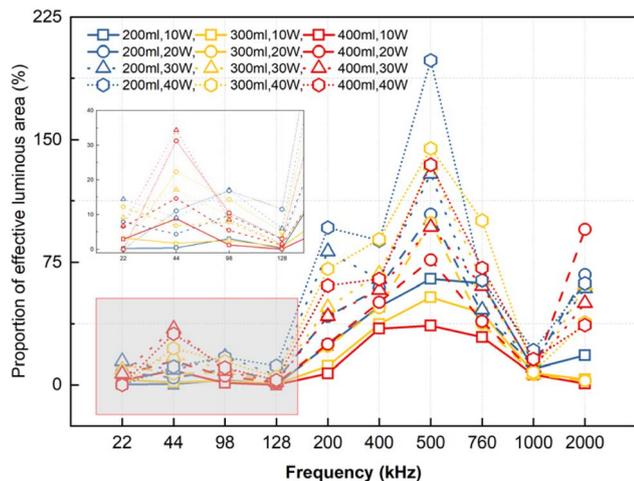
Fig. 10 The variation of effective SCL area with frequency, power, and volume.
