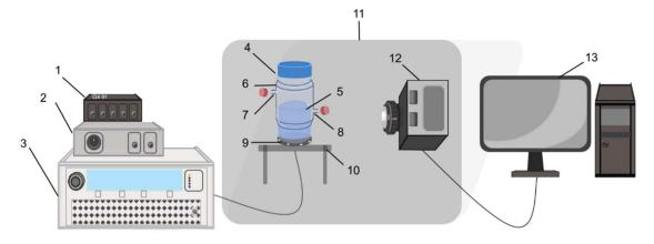
1.Resistor (input powertection) 2.Impedance matching device 3.Amplifier (PF output) 4.Reactor 5.Sample container 6.Cooling jacket 7.Coolant outflow 8.Coolant inflow 9.Transducer (frequency output) 10.Stand 11. Dark box 12.Camera (ANDOR iXon3 EMCCD) 13. Computer
