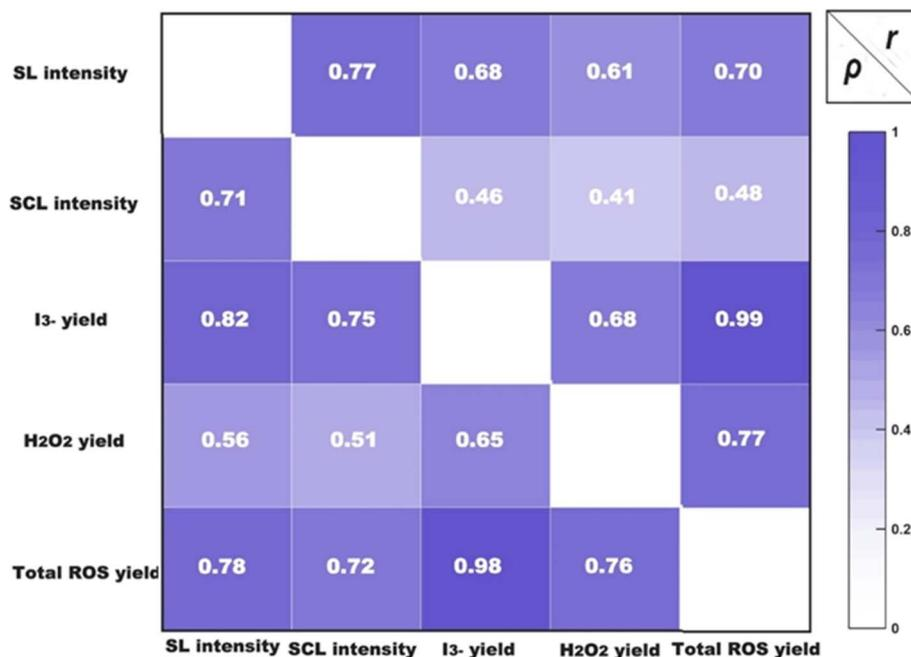
Fig. 15 The correlation coefficients between I<sub>3</sub><sup>-</sup> yield, H<sub>2</sub>O<sub>2</sub> yield, total ROS yield, SL intensity and SCL intensity.
