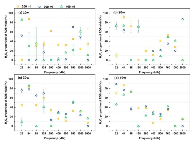
Fig. 13  $H_2O_2$  proportion of total ROS yield with different frequencies and solution volume: (a) 10 W, (b) 20 W, (c) 30 W and (d) 40 W.
