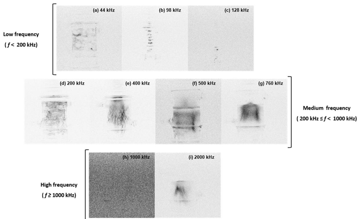
Fig. 6 SCL emission at 40 W loading-power, 400 ml reactor volume, and frequencies with (a–c)  $f < 200$  kHz, (d–g)  $200$  kHz  $\leq f < 1000$  kHz, and (h and i)  $f \geq 1000$  kHz. Image colour-reversal.
