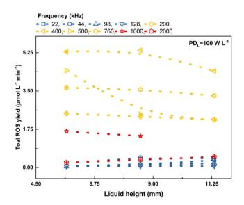
Fig. 14 Correlation between liquid height and ROS yield at different frequencies with same power density (100 W  $\rm L^{-1}$ ).
