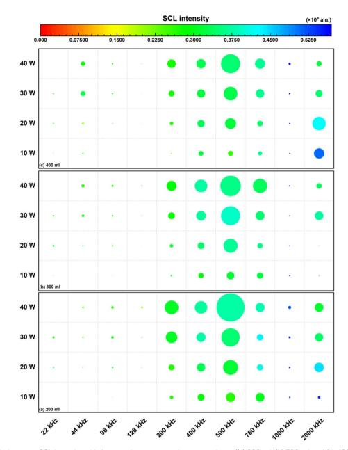
Relationship between SCL intensity with frequencies, power and reactor volume ((a) 200 ml, (b) 300 ml and (c) 400 ml).
