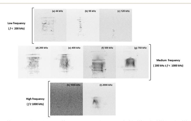
Fig. 6 SCL emission at 40 W loading-power, 400 ml reactor volume, and frequencies with (a-c) f < 200 kHz,  $(d-g) 200 \text{ kHz} \le f < 1000 \text{ kHz}$ , and (h and i)  $f \ge 1000$  kHz. Image colour-reversal.
