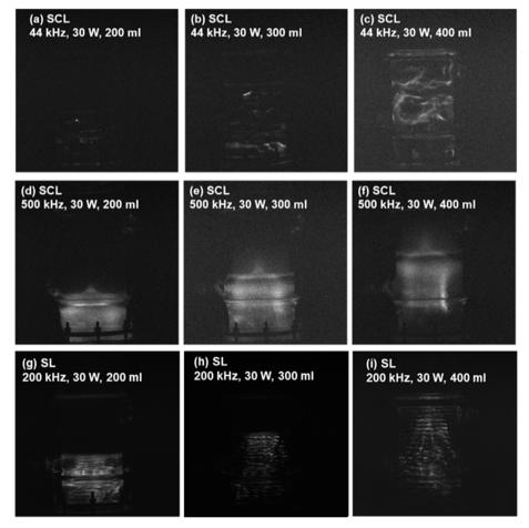
Fig. 11 SCL distribution in different solution volumes under 44 kHz (a-c), 500 kHz (d-f) and 200 kHz (q-i).
