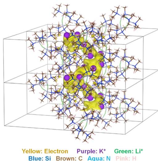
Fig. 6 The AIRSS calculated structure of electride **13**, showing the helical anionic electron density topology.<sup>64</sup>
