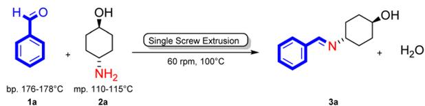
Scheme 4 Synthesis of a cyclohexanol aldimine in a single screw hot melt extruder.
