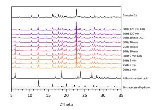
Fig. 2 Comparison between the PXRD traces of the mechanochemical syntheses of 2m under different grinding conditions; the calculated patterns of 2s (top) and of the reagents (bottom) are also reported.
