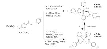
Scheme 1 — The different synthetic paths adopted in this work to obtain zinc complexes: (a) and (c) solution syntheses for complexes 1s-3s and 7s-8s; (b) and (d) mechanochemical syntheses for complexes 1m-3m and 7m-8m (see Experimental for details).
