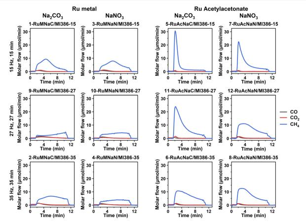
Transient gas profiles of CO, CO<sub>2</sub> and CH<sub>4</sub> during the 5th methanation step (350 °C, 10% H<sub>2</sub>/N<sub>2</sub>, 50 mL min<sup>-1</sup>, and 250 mg).
