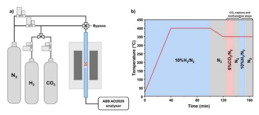
Scheme 1 (a) Reaction apparatus scheme composed of independently controlled mass flow controllers connected to a 4-way valve leading to the reactor or a bypass; (b) ICCU-MET reaction procedure. The  $CO_2$  capture and methanation steps represent one cycle; 5 cycles are performed per experiment.
