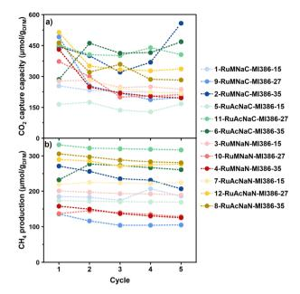
(a) CO<sub>2</sub> capture capacity and (b) CH<sub>4</sub> production for each cycle of the DFMs tested at 350 °C under 5% CO<sub>2</sub>/N<sub>2</sub> and 10% H<sub>2</sub>/N<sub>2</sub> (50  $mL min^{-1}$ , 250 mg, and 10 min each cycle).
