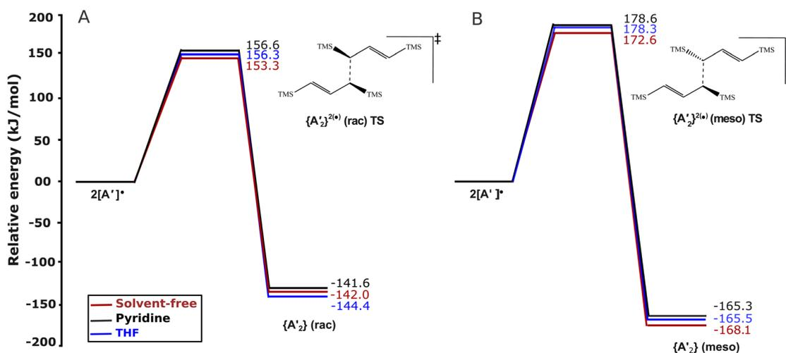
Fig. 5 Energy profile diagram of the synthesis of the  $\{\text{A}'_2\}$  molecule in *rac* (A) and *meso* (B) forms. The solid red, black, and blue lines represent the case without solvent, with pyridine, and with THF, respectively.
