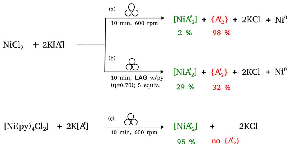
Fig. 1 Reaction schemes for [NiA'<sub>2</sub>] synthesis using (a) neat grinding, (b) liquid-assisted grinding (LAG), and (c) solvate-assisted grinding (SAG).<sup>10</sup> The green and red text represent the experimentally observed yields for [NiA'<sub>2</sub>] and {A'<sub>2</sub>}, respectively.
