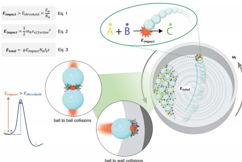
Fig. 3 Illustration of planetary mill kinematics within the jar.<sup>41</sup> Copyright 2024, Wiley-VCH.
