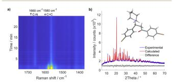
Fig. 1 (a) Time-resolved 2D Raman monitoring of milling 1 and 2a in an equimolar ratio with two ZrO<sub>2</sub> milling balls (mass 1.6 g, diameter 8 mm) in a vibratory ball mill at 30 Hz milling frequency. (b) Experimental diffractogram (blue line) of a powder collected immediately after milling and its Rietveld fit (red line) depicted with the solved crystal structure of 3a (deposited under CCDC number: 2343064).
