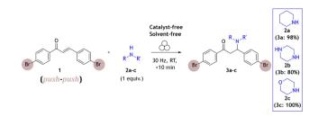
Scheme 1 Mechanochemical aza-Michael addition reaction of secondary cyclic amines 2a-c to chalcone 1 performed in a vibratory ball mill. The yields were evaluated according to the  $^1H$  NMR signals of reactants and the product.
