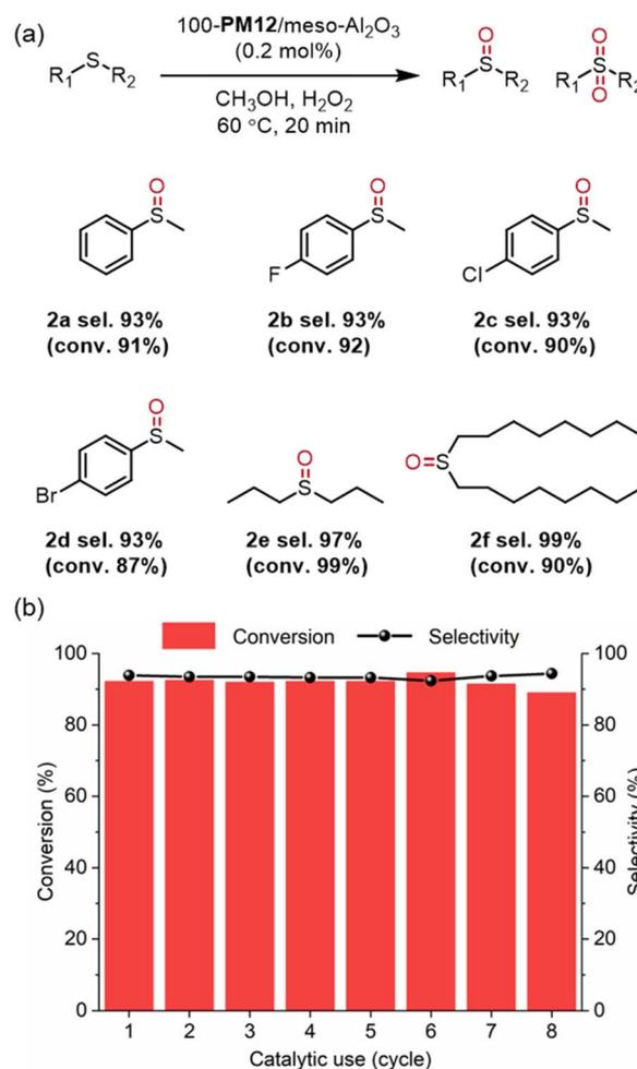
Fig. 3 100-**PM12**/meso-Al<sub>2</sub>O<sub>3</sub>-catalyzed selective oxidation of (a) different sulfide substrates; and (b) reused catalytic tests for selective oxidation of **1a**.
