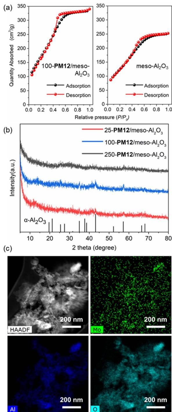
Fig. 2 (a)  $\text{N}_2$  adsorption–desorption isotherms (77 K) of 100-**PM12/meso-Al}\_2\text{O}\_3 and  $\text{meso-Al}_2\text{O}_3$ ; (b) XRD spectra of varying loading amounts of POMs as  $x\text{-PM12/meso-Al}_2\text{O}_3$ ; (c) STEM EDS-mapping images of 100-**PM12/meso-Al}\_2\text{O}\_3.****
