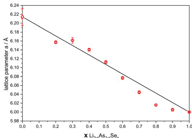
Fig. 5 Lattice parameter  $a$  plotted against the mole fraction  $x$  of the solid solution  $\text{Li}_{3-x}\text{As}_{1-x}\text{Se}_x$  ( $0.2 \leq x \leq 1$ ).
