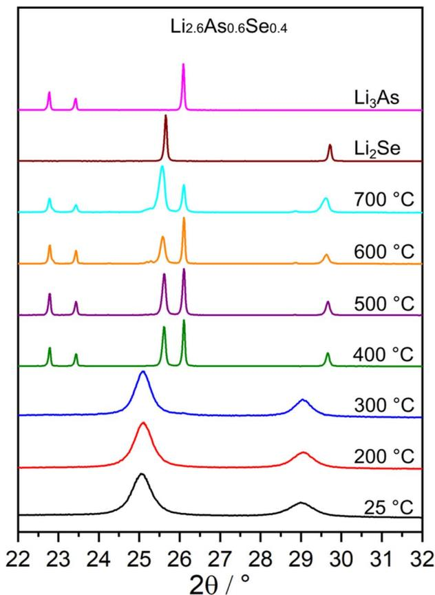
Fig. 7 Powder diffractograms of the  $\text{Li}_{2.6}\text{As}_{0.6}\text{Se}_{0.4}$  compound after annealing to the displayed temperatures for one week and powder diffractograms of the end members  $\text{Li}_3\text{As}$  (hexagonal) and  $\text{Li}_2\text{Se}$ .
