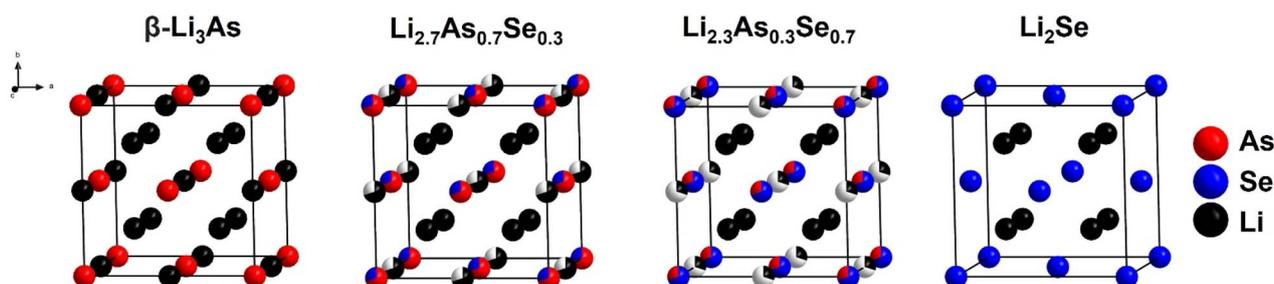
Fig. 6 Structural progression of the solid solution in the system Li<sub>3-x</sub>As<sub>1-x</sub>Se<sub>x</sub> (0.2 ≤ x ≤ 1) with the parent compounds  $\beta$ -Li<sub>3</sub>As and Li<sub>2</sub>Se.
