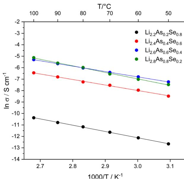
Fig. 8 Arrhenius plot of the solid solution  $\text{Li}_{3-x}\text{As}_{1-x}\text{Se}_x$  ( $0.2 \leq x \leq 1$ ).
