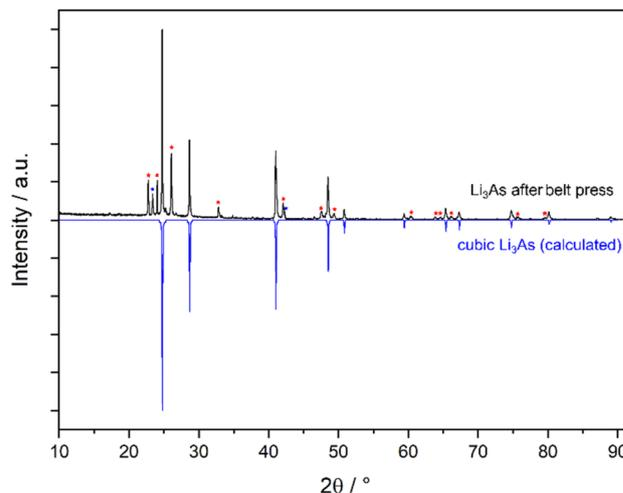
Fig. 1 Powder diffractogram of  $\text{Li}_3\text{As}$  after quenching from high-pressure and temperature to ambient conditions (black). Intensities marked with red stars can be assigned to hexagonal  $\text{Li}_3\text{As}$  (~36%). The intensity marked in blue cannot be assigned to any phase. Negative intensities show the calculated cubic  $\text{Li}_3\text{As}$  modification in the space group  $Fm\bar{3}m$  (no. 225) with lattice parameters determined from the measured diffractogram.
