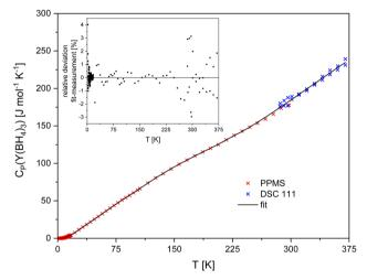
Fig. 2 Temperature dependence of the molar heat capacity  $C_P$  of  $Y(BH_4)_3$  in the temperature range from about 2 K to 370 K. The inset shows the relative deviation of the experimental data from the fit
