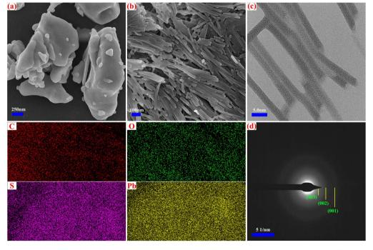
Fig. 1 SEM images of (a) Pb(NO<sub>3</sub>)<sub>2</sub> and (b) Pb(DS)<sub>2</sub>, HRTEM images of (c) Pb(DS)<sub>2</sub>, and the SAED pattern of (d) Pb(DS)<sub>2</sub>, including EDS mapping spectra.
