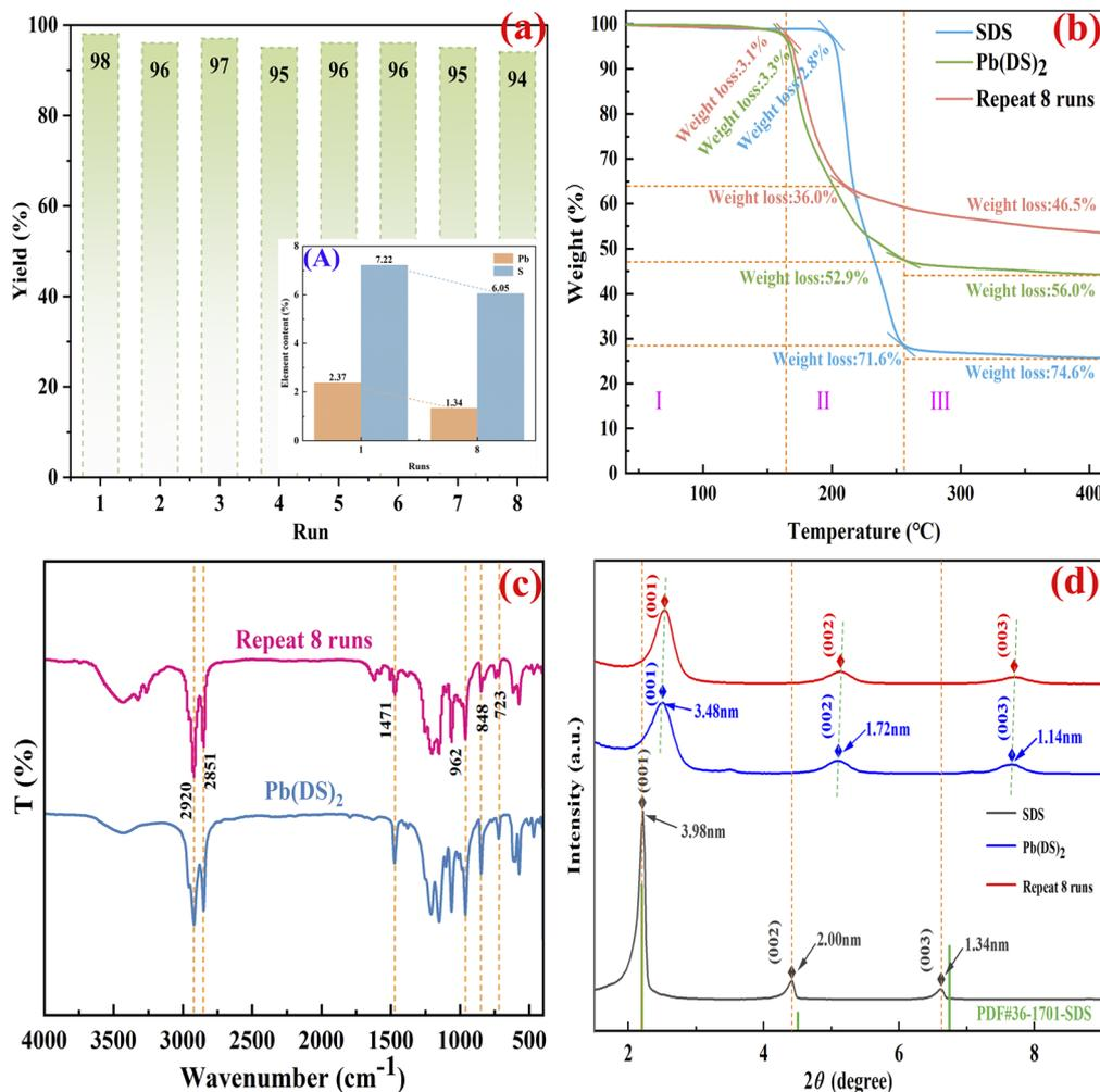
Fig. 4 The experimental evaluation of Pb(DS)<sub>2</sub> recycling (a), elemental analysis of the fresh Pb(DS)<sub>2</sub> catalyst and after 8 runs (A), TGA (b), FT-IR (c) and XRD (d), respectively.
