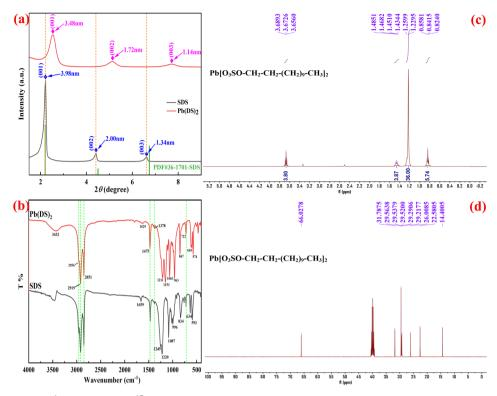
Fig. 2 The XRD (a), FT-IR (b), <sup>1</sup>H-NMR (c), and <sup>13</sup>C-NMR (d) spectra of Pb(DS)<sub>2</sub>, respectively
