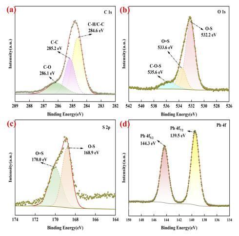
Fig. 3 The XPS of the Pb(DS)<sub>2</sub> catalyst.
