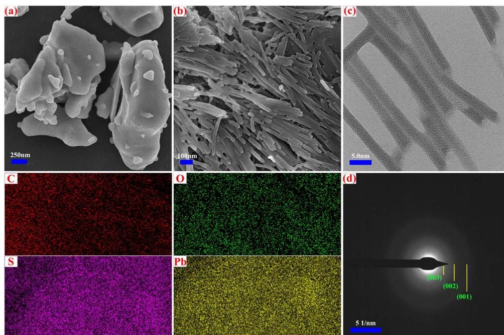
Fig. 1 SEM images of (a)  $\text{Pb}(\text{NO}_3)_2$  and (b)  $\text{Pb}(\text{DS})_2$ , HRTEM images of (c)  $\text{Pb}(\text{DS})_2$ , and the SAED pattern of (d)  $\text{Pb}(\text{DS})_2$ , including EDS mapping spectra.
