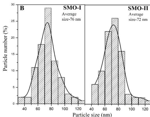
**Fig. 4** Particle size distribution histogram of mechanochemically synthesized SMO-I (5 h/500 rpm) and SMO-II (1 h/850 rpm) samples.
