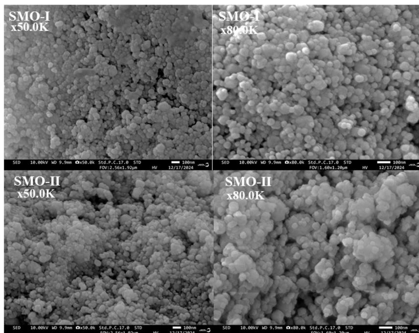
**Fig. 3** SEM micrographs of mechanochemically synthesized SMO-I (5 h/500 rpm) and SMO-II (1 h/850 rpm) samples at different magnifications.
