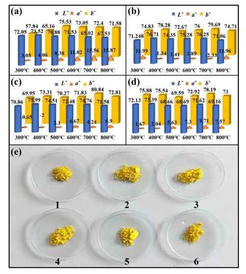
Fig. 2 Color coordinates of MDAPT@BiVO<sub>4</sub> hybrid pigments prepared with different amounts of MDAPT and different calcining temperatures: (a) 20 wt%, (b) 40 wt%, (c) 60 wt%, and (d) 80 wt%). (e) Digital photographs of the hybrid pigments prepared at different calcining temperatures after incorporation of 60 wt% MDAPT.
