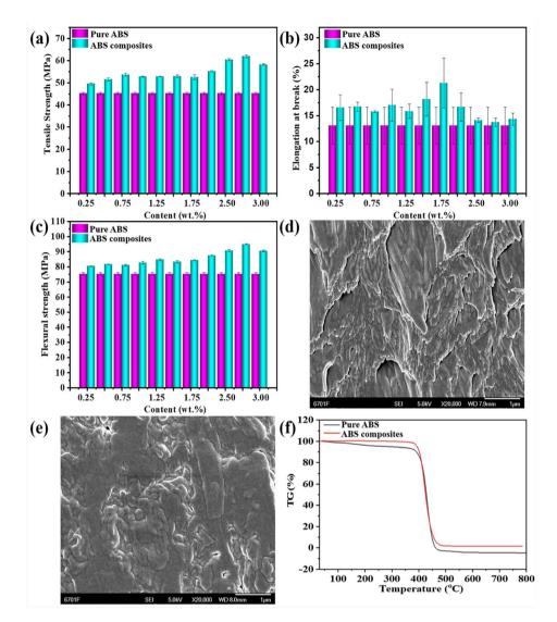
Fig. 7 Effect of the contents of hybrid pigments on the mechanical properties of ABS composites: (a) tensile strength, (b) elongation at break and (c) bending strength. SEM images of the bending failure section for (d) pure ABS and (e) ABS composites, (f) TGA curves of pure ABS and ABS composites.
