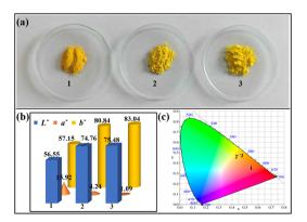
Fig. 5 (a) Digital photographs of the prepared hybrid pigments, the chromaticity values of (b) the pigments and (c) chromaticity CIE coordinate diagram ((1) Raw MDAPT@BiVO $_4$ -700-60, (2) MDAPT@BiVO $_4$ -700-60, (3) KH-570 modified MDAPT@BiVO $_4$ -700-60).
