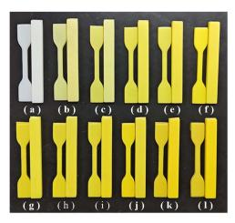
Fig. 6 Tensile and bending splines of ABS composites containing different contents of KH-570 modified MDAPT@BiVO<sub>4</sub>-700-60 ((a): 0.00 wt%, (b): 0.25 wt%, (c): 0.50 wt%, (d): 0.75 wt%, (e): 1.00 wt%, (f): 1.25 wt%, (g): 1.50 wt%, (h): 1.75 wt%, (i): 2.00 wt%, (j): 2.50 wt%, (k): 2.75 wt%, and (l): 3.00 wt%).
