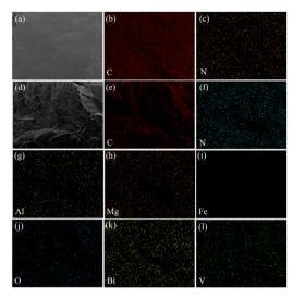
Fig. 8 Elemental mappings of the tensile splines of pure ABS (a-c) and ABS composites containing KH-570 modified MDAPT@BiVO<sub>4</sub>-700-60 (d-l) after bending testing.
