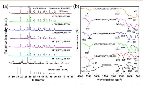
Fig. 3 XRD patterns (a) and FTIR spectra (b) of hybrid pigments prepared at different calcination temperatures after introduction of 60 wt% MDAPT.
