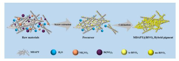
Fig. 1 A schematic diagram of the preparation process of BiVO<sub>4</sub> hybrid pigments
