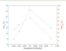
Fig. 2 The calculated degree of substitution of the formed Schiff base (DS<sub>FA</sub>) and reaction mass efficiency (RME<sub>FA</sub>) based on elemental analysis (EA) in function of the added equivalents of citronellal. The chitosan mass within the system was kept constant at 500 mg. A 25 mL SS jar was utilized together with two 15 mm SS balls at a frequency of 30 Hz. The dotted lines connect the different data points and are only added as a guide to the eye.
