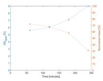
Fig. 4 The degree of substitution (DS<sub>NMR</sub>, calculated based on <sup>1</sup>H NMR) and the percentage of mass that was recovered after the reaction in function of time. The previously explained two-step protocol utilizing NaBH<sub>4</sub> (see entry 6 Table 1) was utilized for all reactions. The dotted lines connect the different data points and are only added as a guide to the eye.
