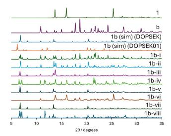
Fig. 4 Powder X-ray diffractograms of products obtained during the optimization of the RAM preparation of **1b**. From top to bottom: experimental PXRD patterns of **1**, **b**, simulated PXRD pattern of **1b** (DOPSEK), simulated PXRD pattern of a known polymorph of **1b** (DOPSEK01), followed by experimental data for attempts **1b-i**, **1b-ii**, **1b-iv**, **1b-v**, **1b-v**, **1b-vi**, **1b-vii** (see Table 3).
