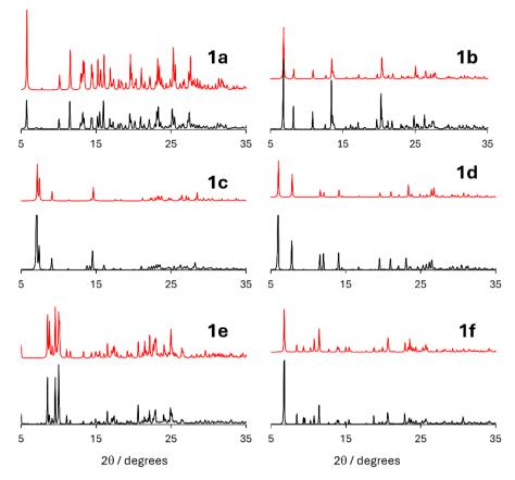
Fig. 6 Experimental (black) and simulated (red) powder X-ray diffractograms for chalcogen-bonded cocrystals 1a, 1b, 1c, 1d, 1e, and 1f. Note that the intensity of the experimental lowest angle reflection for 1c, 1d, and 1f has been truncated for display purposes, i.e., to increase visibility of the lower intensity peaks.
