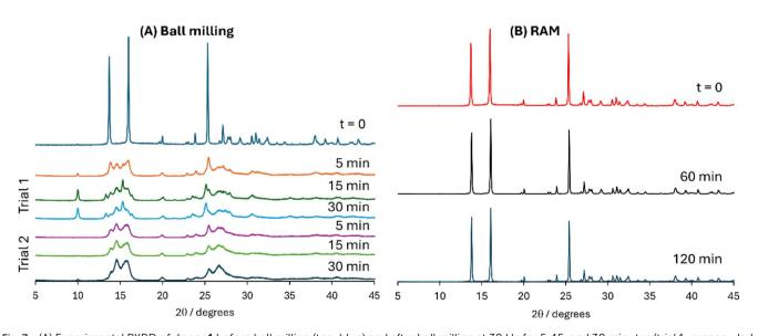
Fig. 7 (A) Experimental PXRD of donor 1 before ball milling (top, blue) and after ball milling at 30 Hz for 5, 15, and 30 minutes (trial 1: orange, dark green, cyan; trial 2: purple, green, dark blue). Amorphization as well as additional peaks indicative of decomposition are seen after five minutes. (B) Experimental PXRD of donor 1 before RAM (top, red) and after RAM at 80g for 60 minutes (black) and 120 minutes (dark blue).
