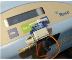
Fig. 2 BOB device interfaced with the Resodyn PharmaRAM I instrument. Left: BOB device (blue box); right: close-up of Servo motor-powered button interacting with the controls of the resonant acoustic mixer.
