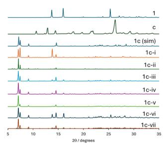
Fig. 5 Powder X-ray diffractograms of products obtained during the optimization of the RAM preparation of 1c. From top to bottom: experimental PXRD patterns for 1, c, simulated PXRD pattern of 1c (SAJPUS), followed by experimental data for attempts 1c-i, 1c-ii, 1c-iii, 1c-iv, 1c-v, 1c-vi, 1c-vii (see Table 4).
