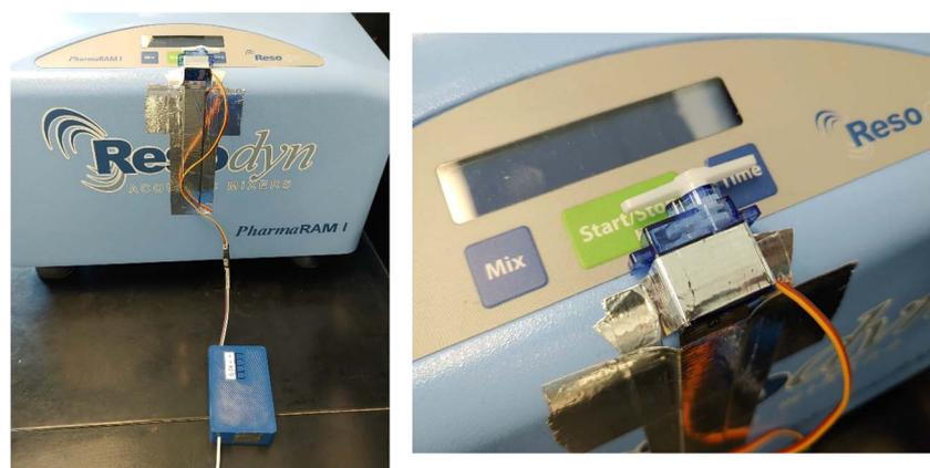
Fig. 2 BOB device interfaced with the Resodyn PharmaRAM I instrument. Left: BOB device (blue box); right: close-up of Servo motor-powered button interacting with the controls of the resonant acoustic mixer.
