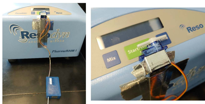
Fig. 2 BOB device interfaced with the Resodyn PharmaRAM I instrument. Left: BOB device (blue box); right: close-up of Servo motor-powered button interacting with the controls of the resonant acoustic mixer.
