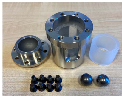
Fig. 1 Milling vessel and 15 mm steel balls used for the in situ XRD experiments. The milling vessel comprises a stainless steel body, equipped with X-ray transparent PMMA windows (shown to the right of the vessel) covering the cut-outs in the steel body.
