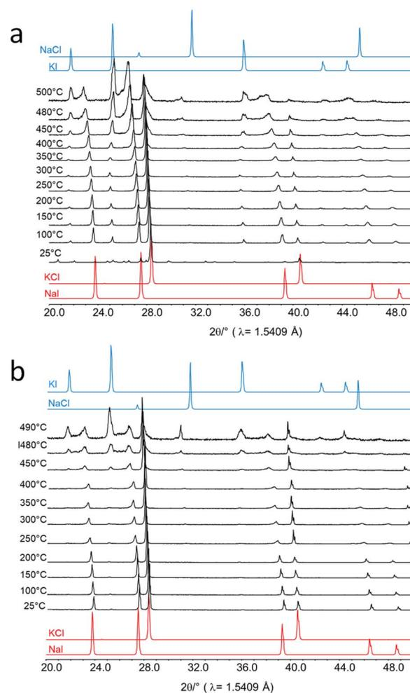
Fig. 7 *In situ* XRD patterns recorded during heating of a physical mixture of NaI and KCl (a) not dried prior to the reaction and (b) dried prior to the reaction. As a reference, simulated diffraction patterns of the educts are shown in red, and those of the products in blue.
