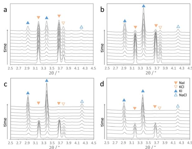
Fig. 2 *In situ* diffraction data of the ion metathesis reaction obtained at shaking frequencies of (a) 15 Hz, (b) 20 Hz, (c) 25 Hz, and (d) 30 Hz using one steel ball and the high energy extension. Time difference of the scans shown is 1 min (scans were recorded continuously for 15 s,  $\lambda = 0.20741$  Å).
