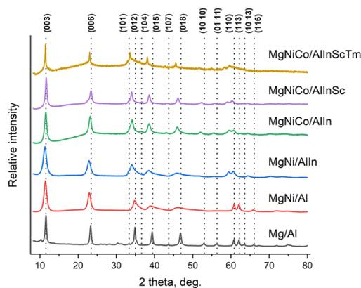
Fig. 1 X-ray diffraction of the LDHs from Mg/Al to MgNiCo/AlInScTm.
