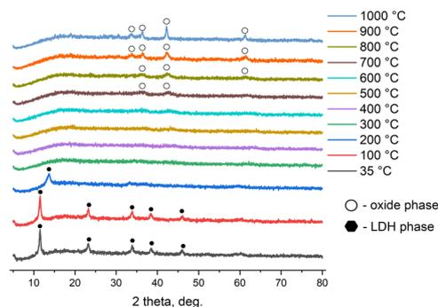
Fig. 7 High-temperature X-ray diffraction of MgNiCo/AlInSc.
