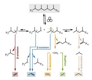
Scheme 1 Proposed examples of mechanistic steps via which  $C_{1-3}$  hydrocarbons are generated during ball milling of PP. Mechanochemical backbone scission forms a primary and a secondary radical which can undergo subsequent radical transfer, hydrogen abstraction, scission, and coupling reactions to form methane, ethane, ethene, propane, and propene.
