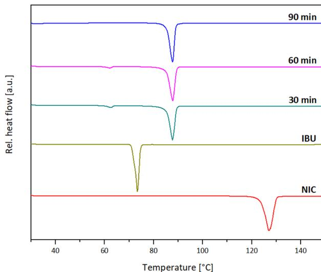
**Fig. 3** DSC measurements for NIC (red, m.p.: 127 °C), IBU (yellow, m.p.: 73 °C), and *rac*-IBU:NIC co-crystal (m.p.: 87–88 °C) formation after 30 min (cyan), 60 min (magenta), and 90 min (blue). LAG additive was added prior to the reaction.
