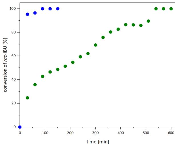
**Fig. 2** Conversion of *rac*-IBU. Green plot: neat grinding approach with addition of 10 kg of balls ( $d = 10$  mm) after 270 min and 10 kg of balls ( $d = 30$  mm) after 360 min; addition of LAG additive EtOH after 510 min. Blue plot: LAG-assisted approach with EtOH added prior to the reaction. The conversion of *rac*-IBU into the *rac*-IBU:NIC co-crystal was determined by the ratio of integrals of NIC and *rac*-IBU in the DSC thermograms (additional DSC data are provided in ESI, Fig. S2†).
