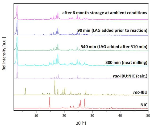
**Fig. 4** PXRD pattern: NIC (red), *rac*-IBU (yellow), calculated *rac*-IBU:NIC co-crystal (purple), reaction after 300 min of neat milling (cyan), final *rac*-IBU:NIC co-crystal product for both approaches (green and blue), and *rac*-IBU:NIC co-crystal after storage for 6 months at ambient conditions (magenta).
