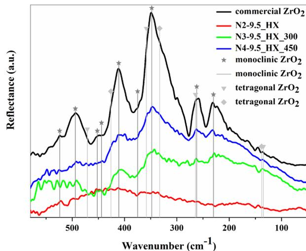
**Fig. 2** Far IR spectra of samples N2-9.5\_HX, N3-9.5\_HXM\_300, N4-9.5\_HXM\_450 and commercial ZrO<sub>2</sub> (reference). The spectra were obtained at 20 °C with an Si window, and polyethylene was used as a background. Marked ★ are the bands of monoclinic ZrO<sub>2</sub> (ref. 71) and ▼ denote bands of tetragonal ZrO<sub>2</sub>,<sup>72</sup> and ◆ bands of tetragonal ZrO<sub>2</sub>.<sup>71</sup>
