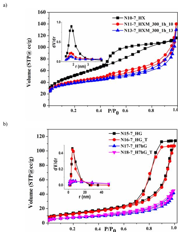
Fig. 5 Nitrogen adsorption-desorption isotherms and PSD curves (insets) for samples of  $ZrO_2$ , precipitated at pH 7, after HTT of the xerogel (a) and gel (b).
