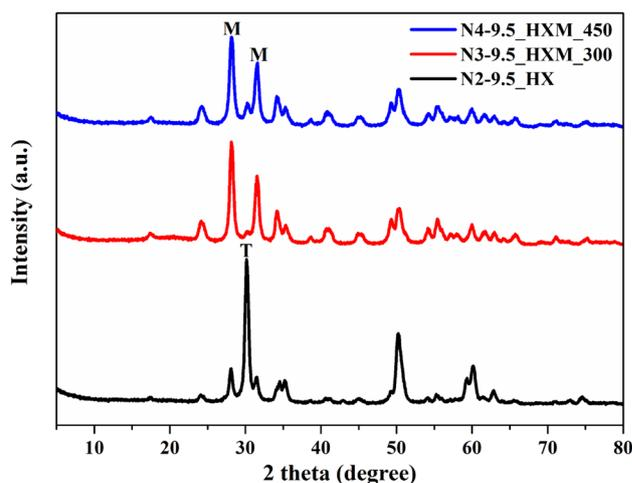
Fig. 1 XRD patterns for ZrO<sub>2</sub>, precipitated at pH 9.5, after HTT and post-milling at 300 and 450 rpm (T – tetragonal phase, peak from plane [101]; M – monoclinic phase, peaks from planes [111] and [–111]).
