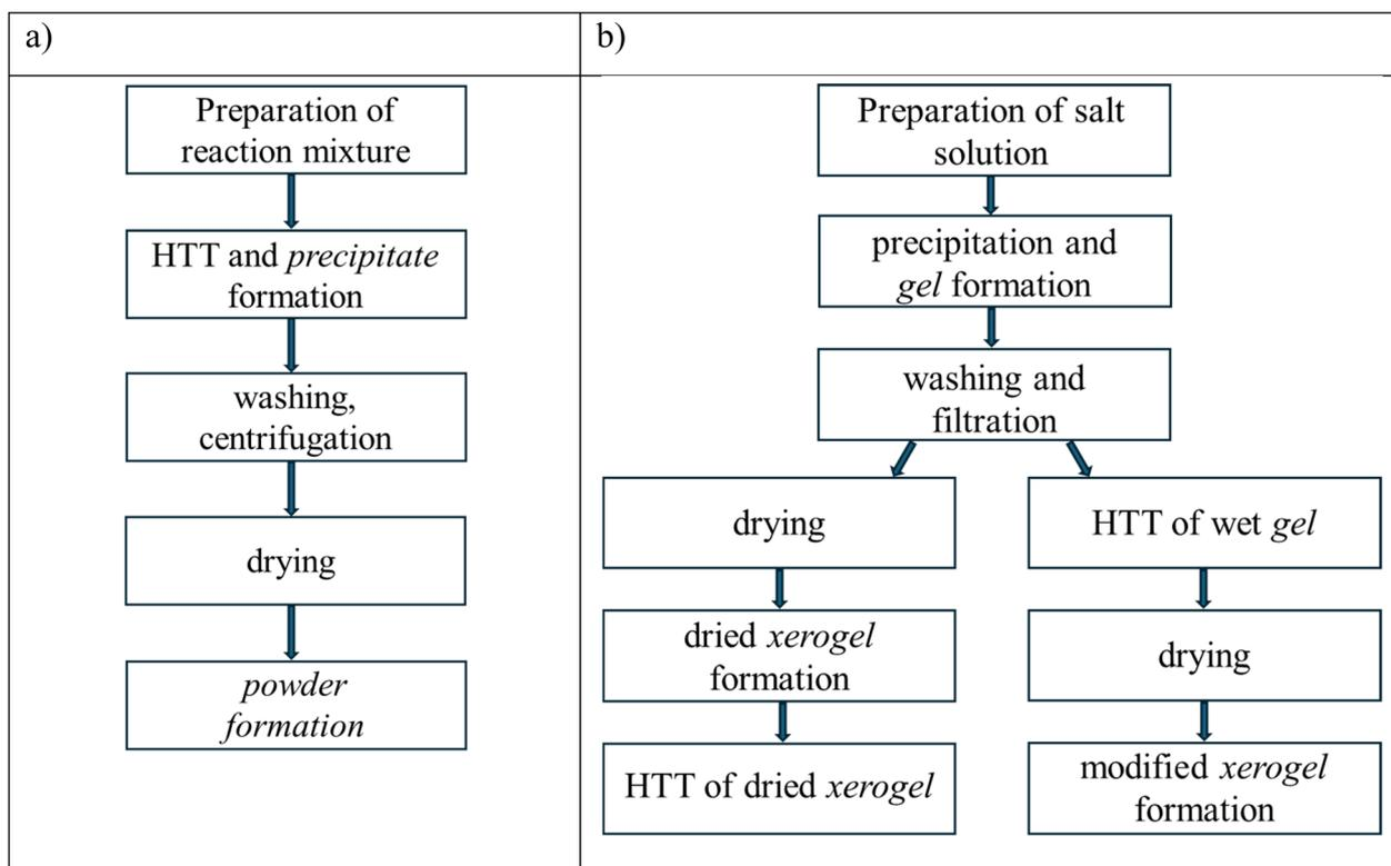
Scheme 1 Preparation of  $ZrO_2$  using procedures (a) previously described and (b) used in this work.
