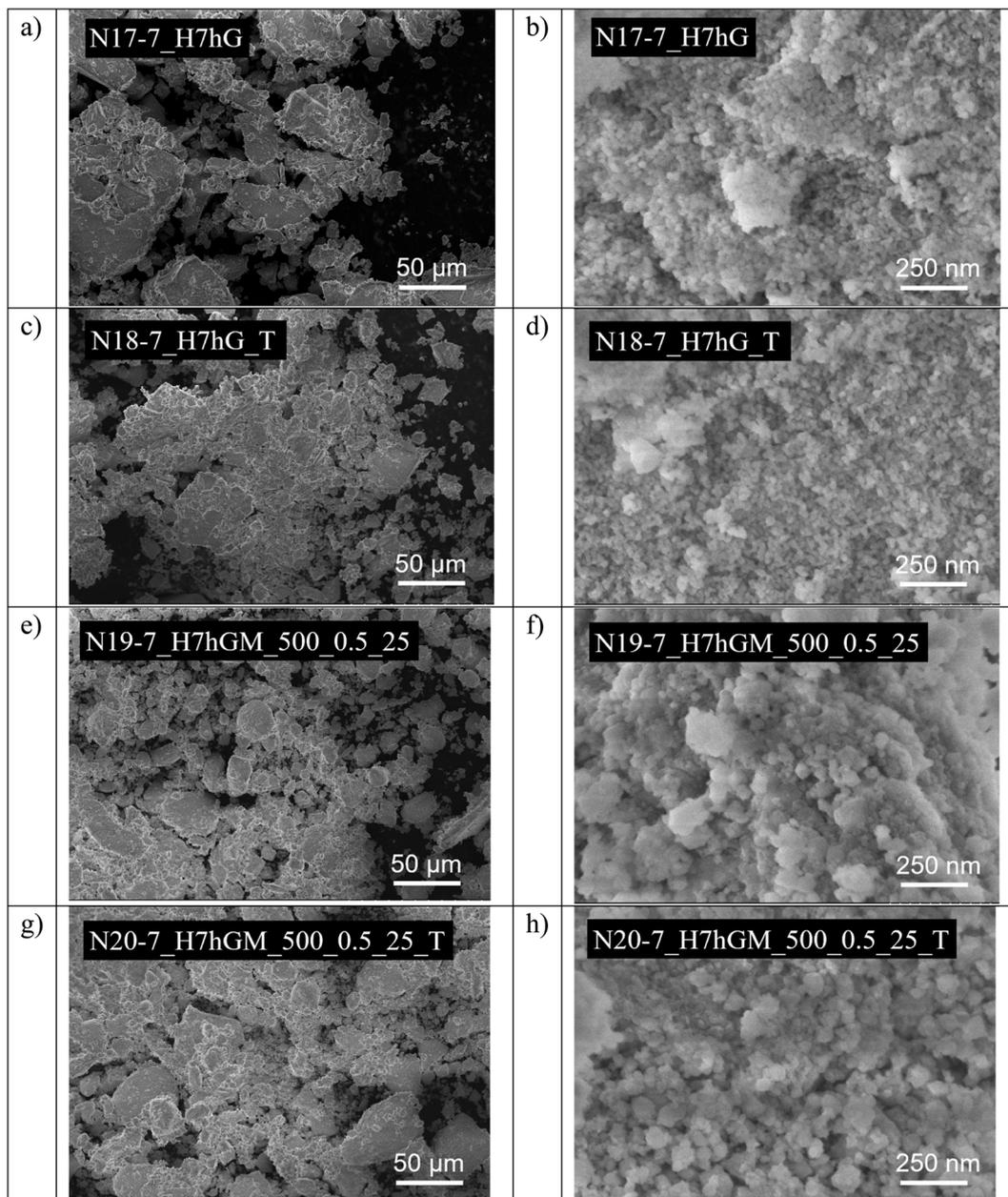
Fig. 7 The effect on the morphology of the hydrothermal sample N17-7\_H7hG (a and b), and its subsequent calcination (c and d), milling (e and f), and post-calcination (g and h).
