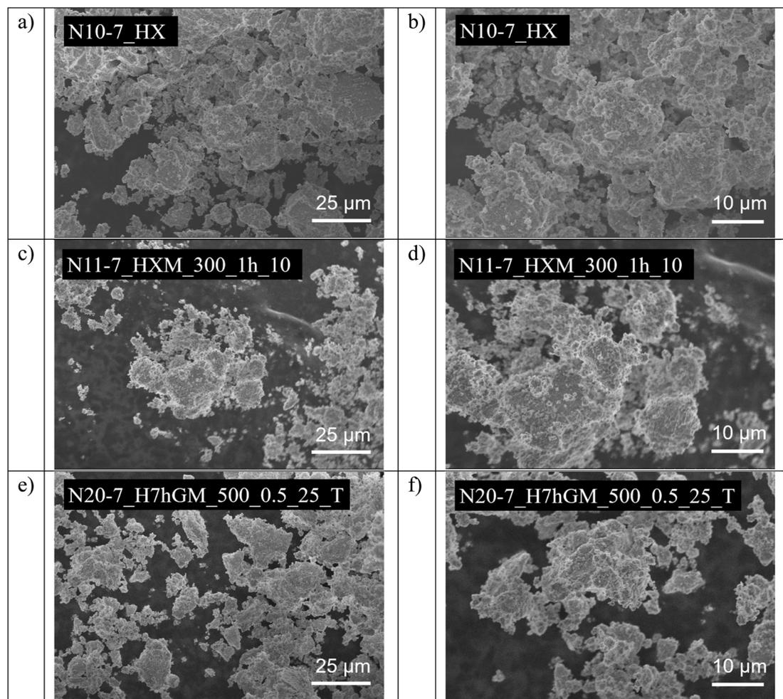
Fig. 6 The effect of different treatments on the morphology of ZrO<sub>2</sub> precipitated at pH 7, samples N10-7\_HX: hydrothermal treatment (a and b), milling (c and d), and post-calcination (e and f).
