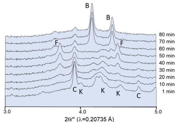
Fig. 8 *In situ* powder patterns collected during milling at 25 Hz. Before milling, 10 drops of absolute ethanol have been added to the jar. F: fairchildite, C: CaCO<sub>3</sub>, B: buetschliite, K: K<sub>2</sub>CO<sub>3</sub>. Intensities are plotted on a square root scale with an offset between the datasets.
