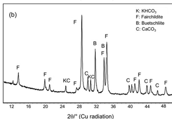
Fig. 4 (a) *Ex situ* X-ray powder patterns of the sample obtained after ball milling at 25 Hz for 60 min of undried educts; bottom data were measured after milling and then every 24 h (192 h total time, upper pattern) under ambient conditions. Intensities are plotted on absolute scale with an offset between the datasets. (b) Final powder pattern collected after 192 h exposure of the sample to ambient conditions.
