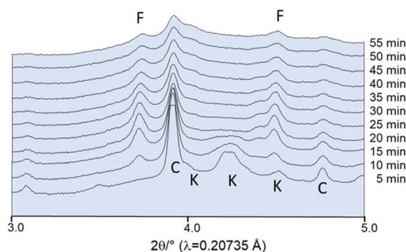
Fig. 9 *In situ* powder patterns collected after milling of dried educts at 25 Hz. F: fairchildite, C: CaCO<sub>3</sub>, K: K<sub>2</sub>CO<sub>3</sub>. Intensities are plotted on a square root scale with an offset between the datasets.
