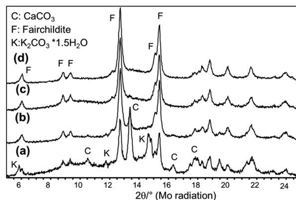
Fig. 5 *Ex situ* X-ray powder patterns obtained after milling of dried educts for (a) 60 min at 25 Hz, (b) 60 min at 30 Hz, (c) 90 min at 30 Hz, and (d) 120 min at 30 Hz. Intensities are plotted on an absolute scale with an offset between the datasets.
