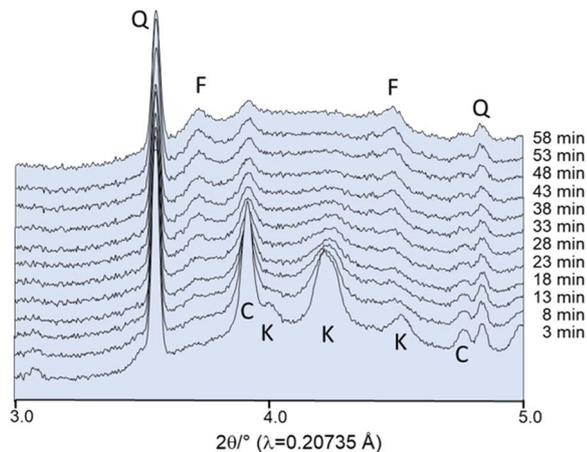
Fig. 6 *In situ* X-ray powder pattern collected during milling at 25 Hz: F: fairchildite, C: CaCO<sub>3</sub>, K: K<sub>2</sub>CO<sub>3</sub>, Q: quartz. Intensities are plotted on a square root scale with an offset between the datasets.
