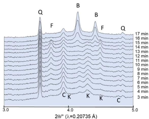
Fig. 7 *In situ* powder pattern collected during milling at 27 Hz: F: fairchildite, C: CaCO<sub>3</sub>, B: buetschliite, K: K<sub>2</sub>CO<sub>3</sub>, Q: quartz. Intensities are plotted on a square root scale with an offset between the datasets.
