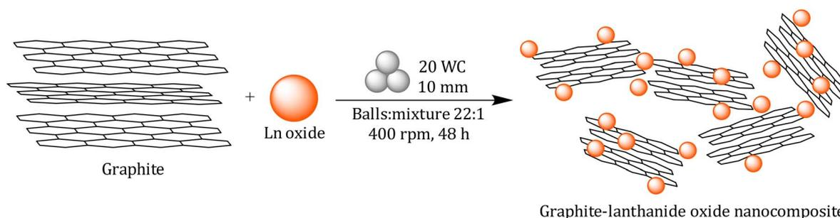
Fig. 1 Mechanochemical preparation of graphite-lanthanide oxide nanocomposites.
