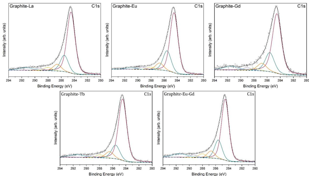
**Fig. 4** Comparison of the C 1s core level spectra of graphite-Ln nanocomposites and the corresponding fits. The components are the same as in Fig. 3 – for details see text.
