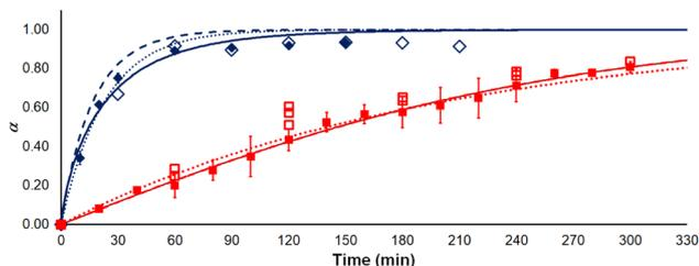
Fig. 4 Compound **5** can also be prepared by  $\eta = 0.5$  EtOH LAG ( $\blacklozenge$ ,  $\diamond$ ) and with the addition of  $\text{Na}_2\text{CO}_3$  to the neat reaction mixture ( $\blacksquare$ ,  $\square$ ). Data shown for reaction mixtures sampled once ( $\diamond$ ,  $\square$ ) and those sampled multiple times ( $\blacklozenge$ ,  $\blacksquare$ ). JMYK (solid lines), FW (dashed lines), and first order modelling (dotted lines) shown.
