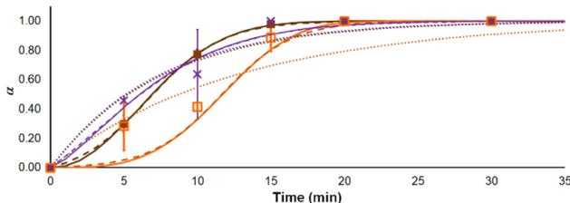
Fig. 3 Measured conversion in mechanochemistry of 2 is affected by sampling. Hand-mixing at 5 min intervals but sampling only once ( $\times$ ) gives similar results to sampling reaction mixtures multiple times ( $\blacksquare$ ). Combining the results of 15 reactions each sampled once gives conversion obtained solely through milling ( $\square$ ). JMYK (solid lines), FW (dashed lines), and first order modelling (dotted lines) shown.
