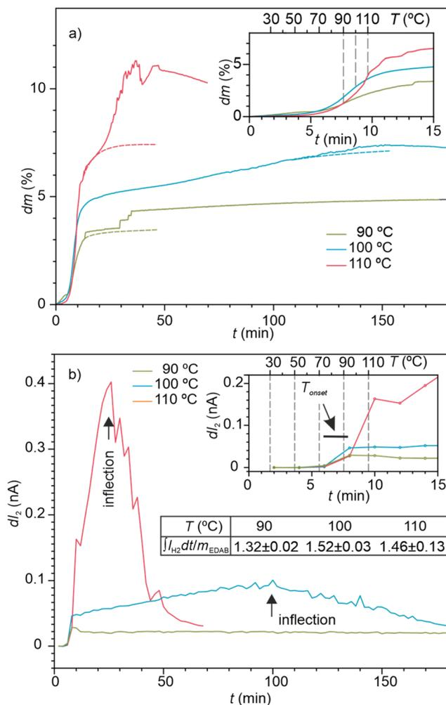
Fig. 6 The results of isothermal TGA-MS at 90 °C, 100 °C and 110 °C: (a) relative mass decrease, (b) variation of  $H_2$  partial pressure. The dashed lines in (a) depict the expected behaviours without foaming and bubbling.
