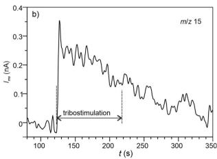
Fig. 2 Representative time series of mass spectrometric signals: (a) coupled behaviour showing continued emission throughout the tribostimulation; (b) uncoupled behaviour, which is triggered by the very first rubbing cycles. After the end of rubbing the signal decays gradually.
