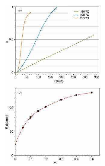
Fig. 7 (a)  $\alpha$ -Time plots of the first step of EDAB decomposition, (b) activation energy for the first-step hydrogen emission obtained for various values of  $\alpha$  using the isoconversional method. The red line is interpolation of the measured data using a fifth-degree polynomial function. The dashed line depicts the possible extrapolated trend of the data towards  $\alpha = 0$ .
