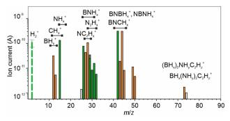
Fig. 1 Mean differential mass-spectrum (DMS) of volatile products emitted from EDAB pellets subjected to rubbing under vacuum at room temperature. The species following coupled and uncoupled behaviours are highlighted in orange and green, correspondingly.
