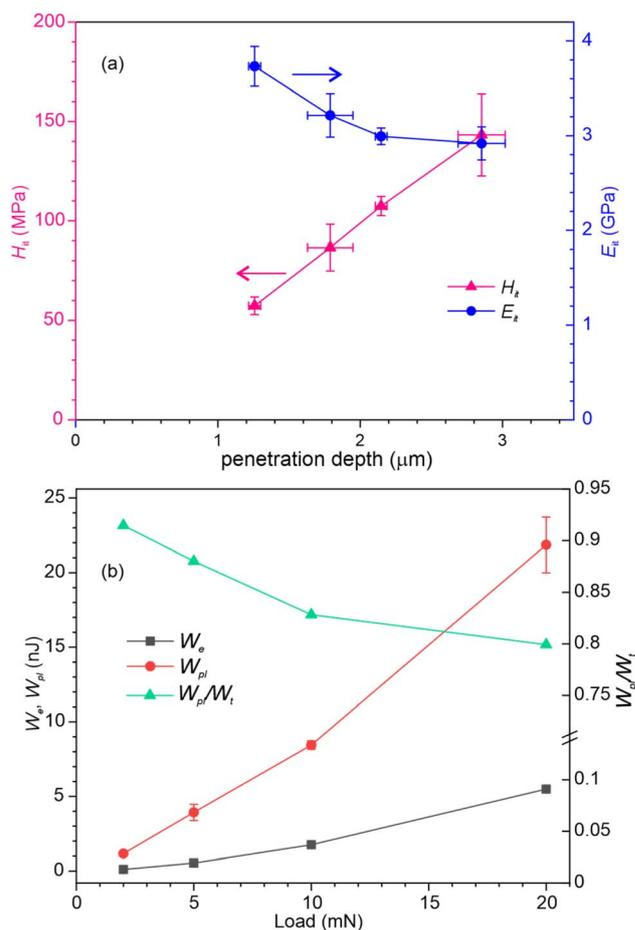
Fig. 5 (a) Hardness and instrumental elastic modulus obtained from nanoindentation tests as function of the penetration depth. (b) Elastic,  $W_e$ , and plastic,  $W_{pl}$ , work expended during nanoindentation of EDAB pellets and corresponding plasticity index.
