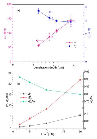
Fig. 5 (a) Hardness and instrumental elastic modulus obtained from nanoindentation tests as function of the penetration depth. (b) Elastic,  $W_{\rm e}$ , and plastic,  $W_{\rm pl}$ , work expended during nanoindenation of EDAB pellets and corresponding plasticity index.
