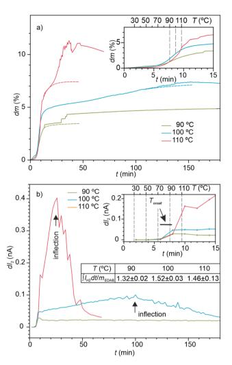
Fig. 6 The results of isothermal TGA-MS at 90 °C, 100 °C and 110 °C: (a) relative mass decrease, (b) variation of H<sub>2</sub> partial pressure. The dashed lines in (a) depict the expected behaviours without foaming and bubbling
