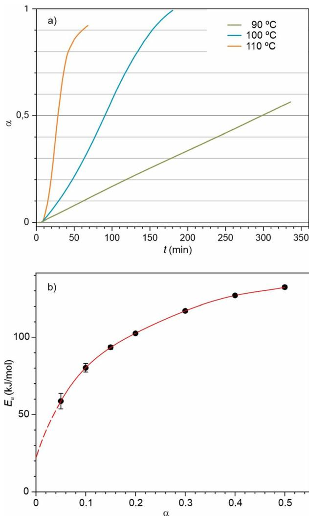
Fig. 7 (a)  $\alpha$ -Time plots of the first step of EDAB decomposition, (b) activation energy for the first-step hydrogen emission obtained for various values of  $\alpha$  using the isoconversional method. The red line is interpolation of the measured data using a fifth-degree polynomial function. The dashed line depicts the possible extrapolated trend of the data towards  $\alpha = 0$ .
