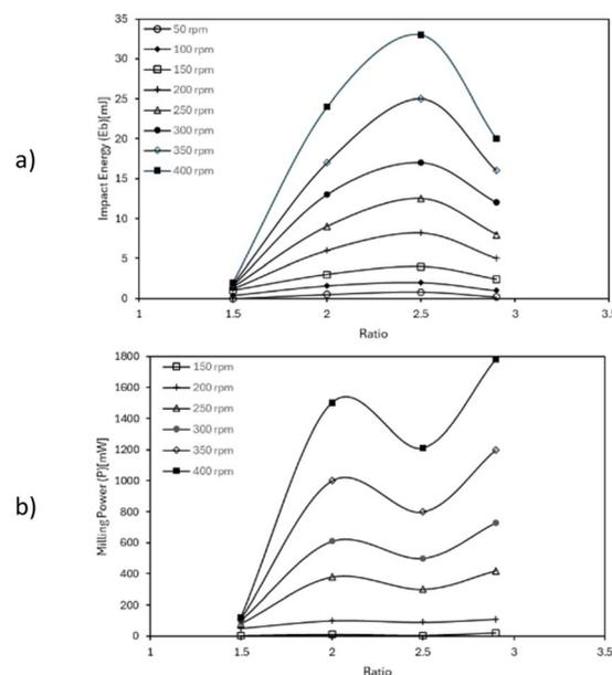
Fig. 2 (a) Impact energy using validated kinematic model<sup>6</sup> with different sun disc speeds and the relationship of the speed ratio between the sun disc and vials. Please note that the rotation of the vials was counter to the sun disc rotation and thus  $W_v$  would be negative. (b) Shows how the milling power would change using the same parameters.
