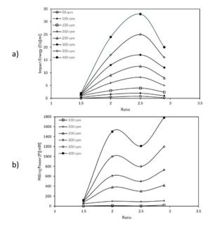
Fig. 2 (a) Impact energy using validated kinematic model<sup>6</sup> with different sun disc speeds and the relationship of the speed ratio between the sun disk and vials. Please note that the rotation of the vials was counter to the sun disk rotation and thus  $W_{\nu}$  would be negative. (b) Shows how the milling power would change using the same parameters.
