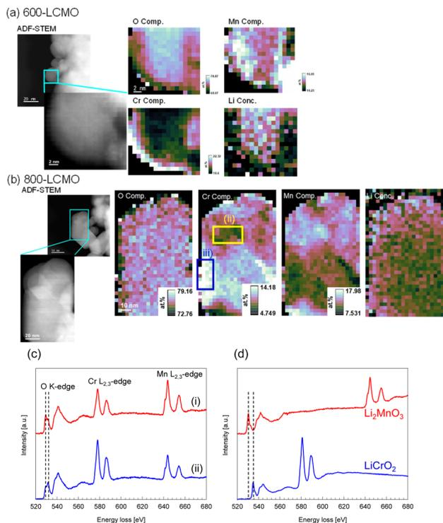
Fig. 4 Image diagrams based on STEM-EELS elemental mapping results for (a) 600-LCMO (EELS spectra for region (i) are shown) and (b) 800-LCMO. (c) EELS spectra for regions (ii), (iii) and (d) and  $\text{LiCrO}_2$  and  $\text{Li}_2\text{MnO}_3$  as standard samples.
