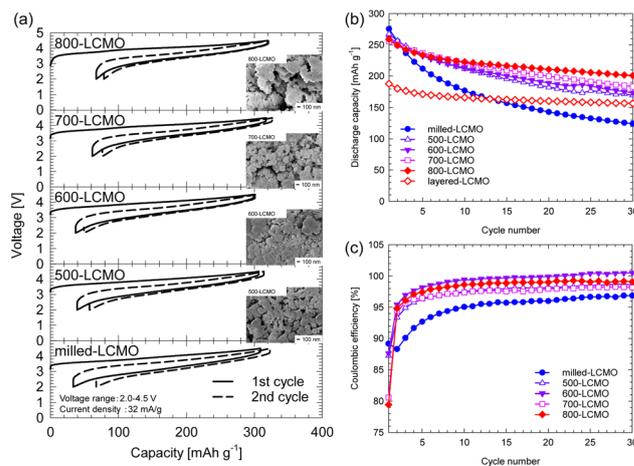
Fig. 5 (a) SEM image and initial and second charge–discharge profiles for thermally treated LCMO, obtained at a rate of  $32 \text{ mA g}^{-1}$  between 2.0 and 4.5 V. (b) Cyclability and (c) coulombic efficiency of the obtained samples.
