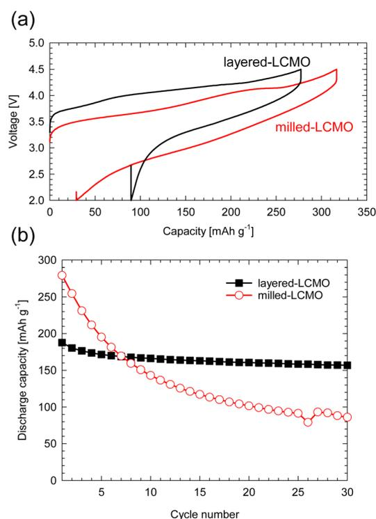
Fig. 1 (a) Initial and second charge–discharge profiles and (b) cyclability of milled-LCMO and layered-LCMO at a rate of  $16 \text{ mA g}^{-1}$  between  $2.0$  and  $4.5 \text{ V}$ .
