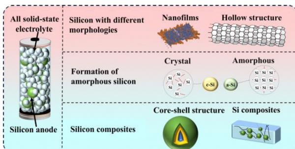
**Silicon anode modification strategies in solid-state lithium-ion batteries**
