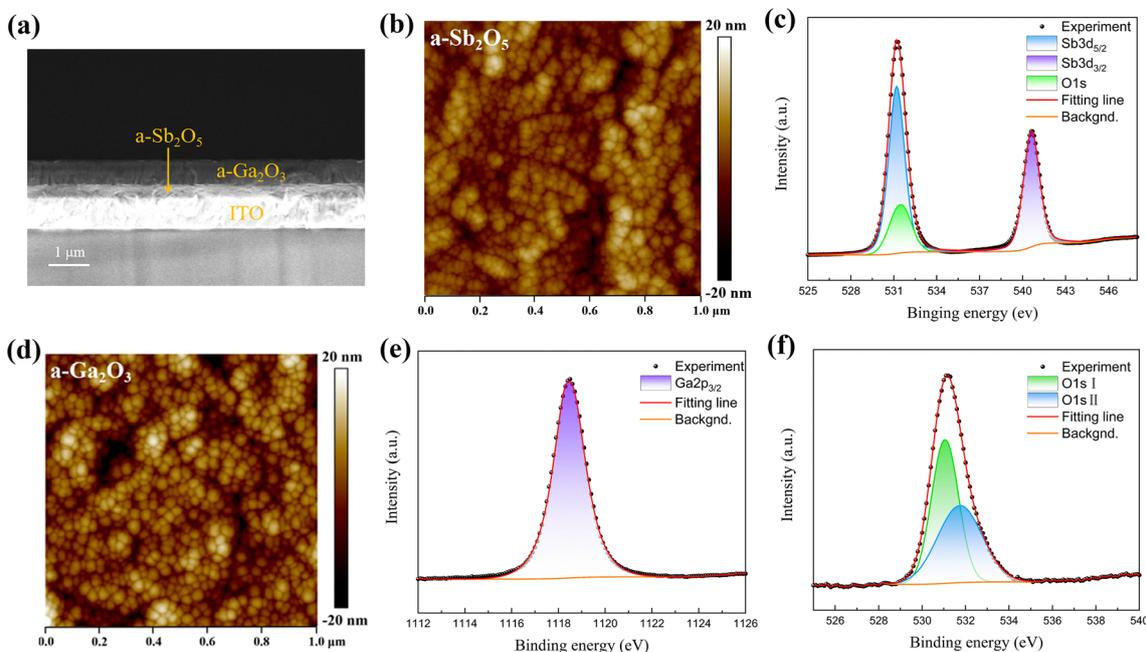
Fig. 1 Morphology and structural characterization of Sb<sub>2</sub>O<sub>5</sub>/a-Ga<sub>2</sub>O<sub>3</sub> heterojunctions. (a) SEM image of the interface of the a-Sb<sub>2</sub>O<sub>5</sub>/a-Ga<sub>2</sub>O<sub>3</sub> heterojunction. (b) AFM image of a-Sb<sub>2</sub>O<sub>5</sub>. (c) XPS image of a-Sb<sub>2</sub>O<sub>5</sub>. (d) AFM image of a-Ga<sub>2</sub>O<sub>3</sub>. (e) and (f) XPS images of a-Ga<sub>2</sub>O<sub>3</sub>.
