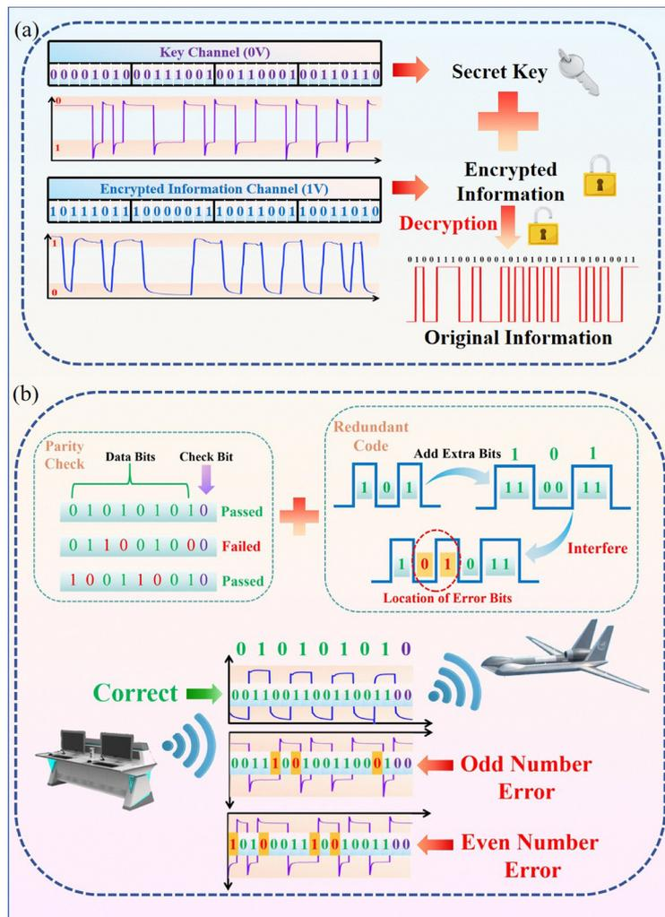
Fig. 6 Two communication modes of a bipolar optical communication system. (a) Real-time encryption mode in an optical communication system. (b) Anti-interference and error correction mode in an optical communication system.
