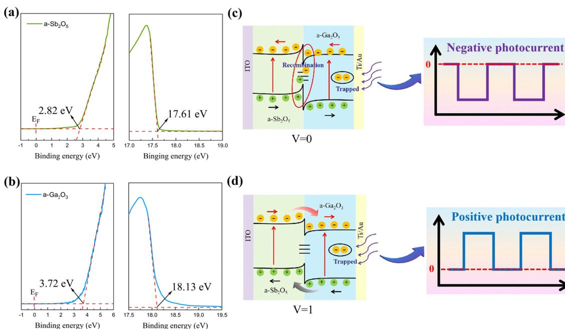
Fig. 4 Schematic diagram of the energy bands and interfacial carrier transfer mechanism of the a-Sb<sub>2</sub>O<sub>5</sub>/a-Ga<sub>2</sub>O<sub>3</sub> bipolar detector. (a) UPS spectrum of a-Sb<sub>2</sub>O<sub>5</sub> (b) UPS spectrum of a-Ga<sub>2</sub>O<sub>3</sub>. (c) NPC response mechanism of the detector under 0 V. (d) PPC response mechanism of the detector under 1 V.
