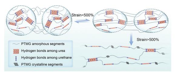
Fig. 21 Proposed mechanism of enhanced puncture resistance, tear resistance, tensile strength, and toughness of CPUU-FA. Reproduced from ref. 165 with permission from John Wiley and Sons, Copyright [2025]
