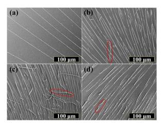
Fig. 9 Fracture surface morphology of (a) EP<sub>0</sub>, (b) EP<sub>2.5</sub>, (c) EP<sub>5</sub> and (d) EP7.5. Reproduced from ref. 63 with permission from Elsevier, Copyright [2023]
