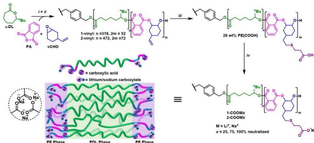
Fig. 17 Synthesis of polyester ionomers. Reproduced from ref. 115 with permission from American Chemical Society, Copyright [2022].
