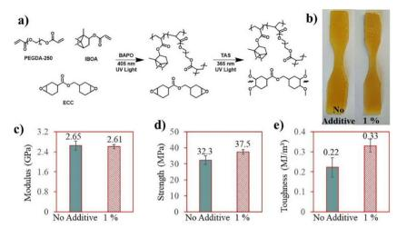
Fig. 3 (a) ECC/IBOA 60:40 wt/wt mixed resin and its blends with the BCP (1 wt%), (b) DLP printed dog bone samples of the ECC/IBOA mixed resin, (c) modulus, (d) failure strength and (e) toughness of the cured samples (p value is 0.033). Reproduced from ref. 32 with permission from Elsevier, Copyright [2023].
