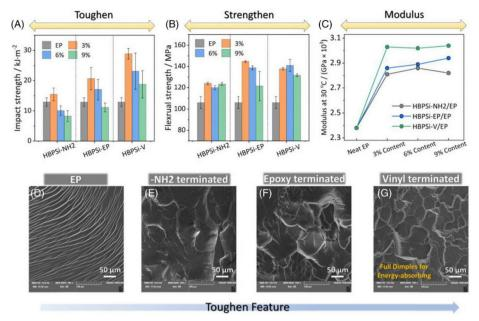
Fig. 10 The mechanical performance test of (A) impact strength, (B) flexural strength, and (C) modulus at 25 °C; (D)–(G) SEM photographs indicate the impact tough facture from native EP to HBPSi-NH2/EP, HBPSi-EP/EP, HBPSi-V/EP. Reproduced from ref. 71 with permission from John Wiley and Sons, Copyright [2023].
