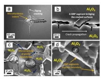
Fig. 4 (a) SEM image of a microhardness indent showing the crack lengths and zigzag failure patterns, (b) the GNP crack-bridging toughening phenomenon, (c) low magnification SEM image of the A4Z fractured surface showing the grain boundary cracks (marked by blue arrows) and (d) the high-magnification SEM image showing well bonded matrix grains in the A4Z0.5G hybrid nanocomposite. Reproduced from ref. 34 with permission from Elsevier, Copyright [2020].
