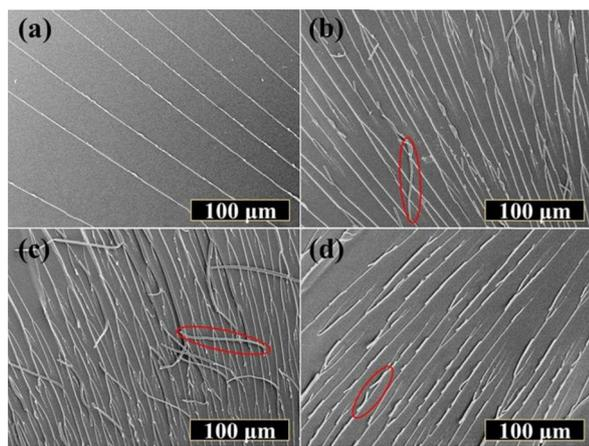
Fig. 9 Fracture surface morphology of (a) EP<sub>0</sub>, (b) EP<sub>2.5</sub>, (c) EP<sub>5</sub> and (d) EP<sub>7.5</sub>. Reproduced from ref. 63 with permission from Elsevier, Copyright [2023].
