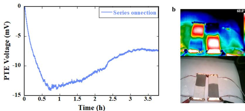
Fig. 3 (a) Voltage profile of two PTE cells connected in series under  $850 \text{ W m}^{-2}$ . (b) Temperature gradient induced in the connected system and the digital photograph of the connected cells.
