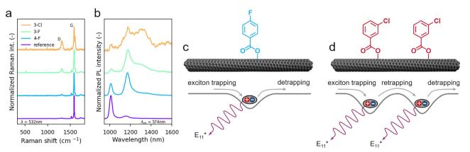
Fig. 5 (a) Raman spectra of pristine SWCNTs and modified with 3-Cl-BPO, 3-F-BPO, and 4-F-BPO, (b) corresponding PL spectra normalized to the intensity of the maximum of the peak of the highest intensity, SWCNT reacted with (c) 4-F-BPO, and (d) 3-Cl-BPO with the schematics of the main phenomena related to exciton dynamics in SWCNTs modified with luminescent defects
