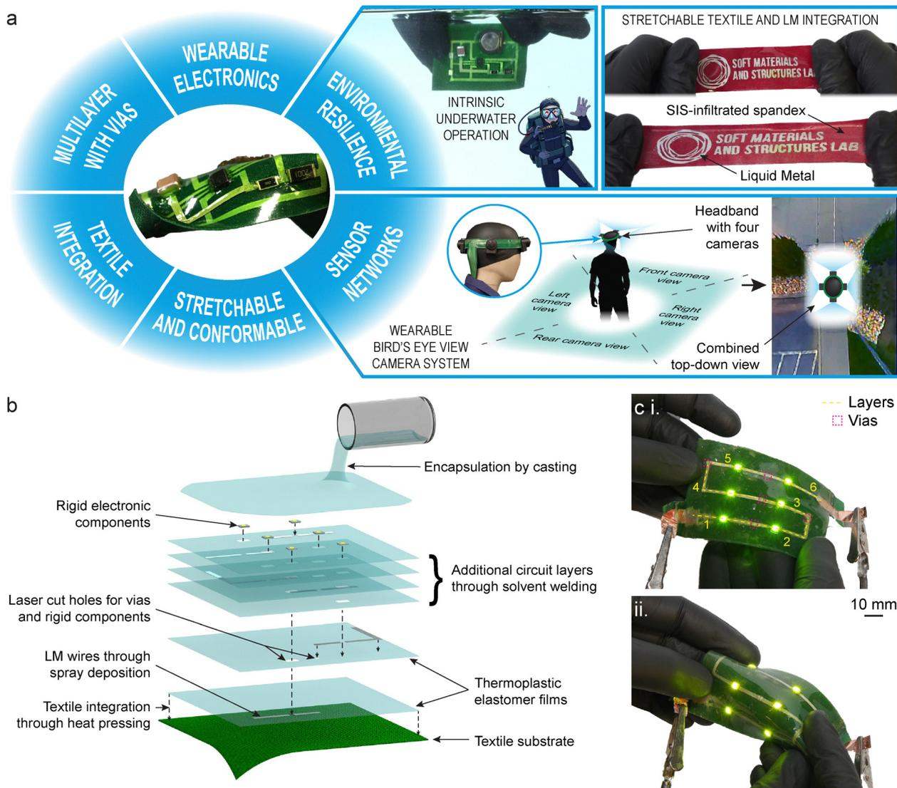
**Fig. 1** Overview of textile-integrated LM soft circuits. (a) Capabilities enabled for wearable electronics, including intrinsic underwater operation (top center), stretchability (top right), and a wearable bird's eye view camera system (second row). (b) Layup of a multilayer textile-integrated LM soft circuit with rigid components embedded. (c) Images of a circuit with six LEDs in series, where each is on a different layer with a via between, in its (i) normal state and (ii) folded.
