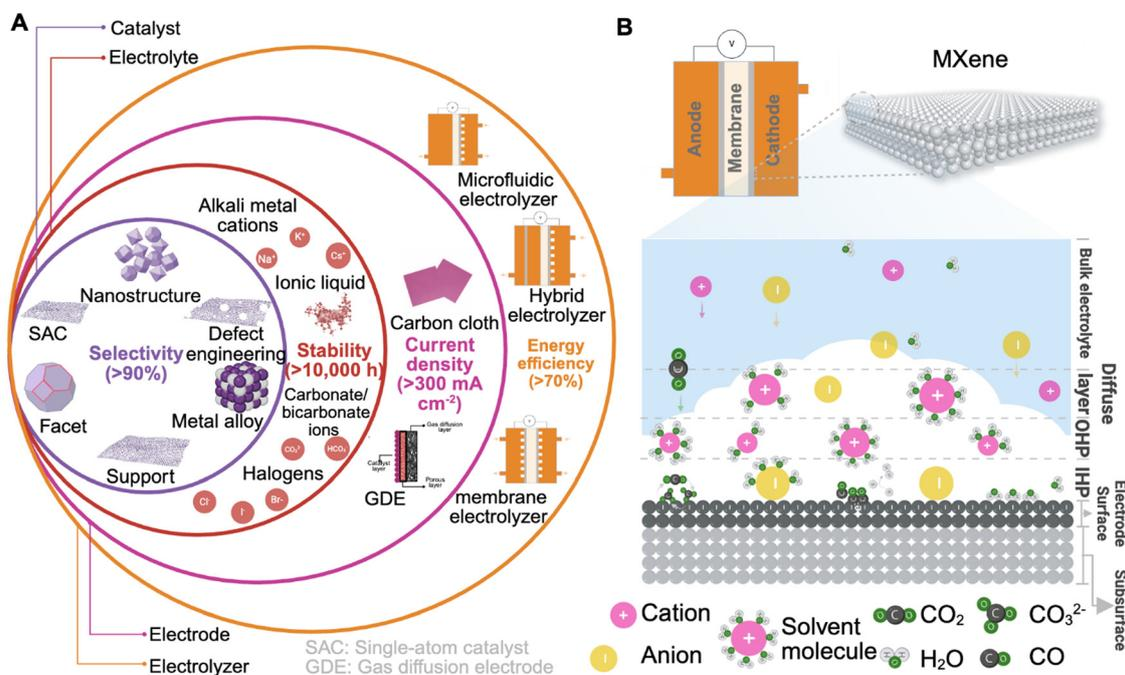
Fig. 3 (A) Factors affecting the  $\text{CO}_2$  electroreduction process. (B) Schematic of the electrode–electrolyte interface for the  $\text{CO}_2\text{RR}$ , accounting for the electric double layer and bulk electrolyte.
