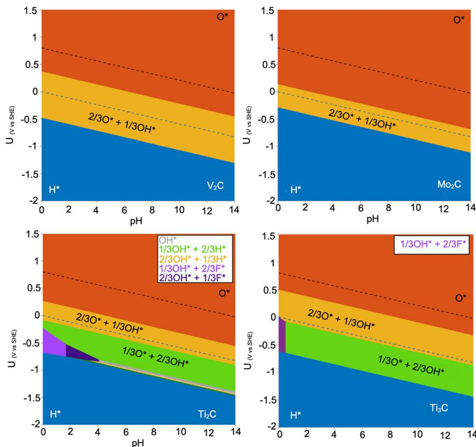
Fig. 5 Pourbaix diagrams of Mo<sub>2</sub>C, V<sub>2</sub>C, Ti<sub>2</sub>C, and Ti<sub>3</sub>C<sub>2</sub>. Reproduced from ref. 91 with permission from Wiley and Sons, Copyright [2022].
