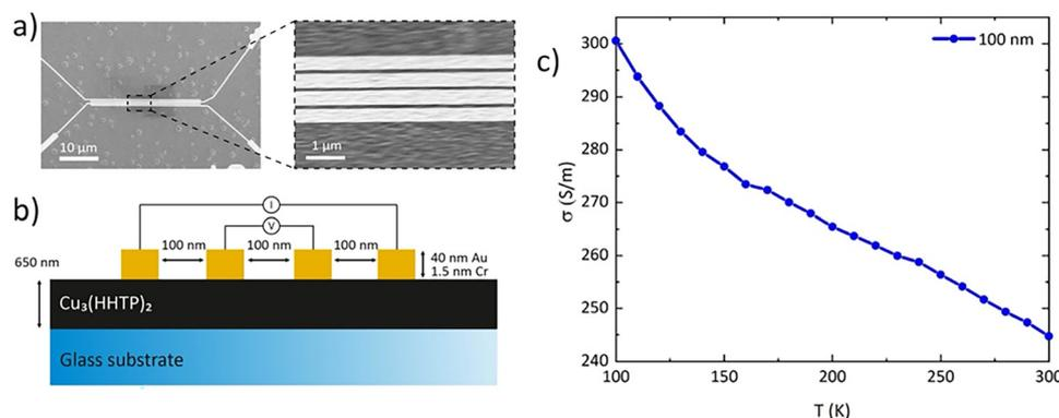
**Fig. 4** (a) Scanning electron microscopy image of a contacted for  $\text{Cu}_3(\text{HHTP})_2$  SURMOF. (b) Schematic of experimental setup used for charge transport measurements (c) experimental electrical conductivities ( $\sigma$ ) measured using a 4-point method for  $\text{Cu}_3\text{HHTP}_2$  SURMOFs with a thickness of 650 nm. The distance between the contacts amounts to 100 nm.
