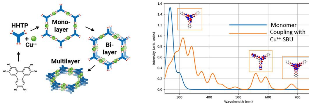
**Fig. 1** Left: Structure of the  $\text{Cu}_3(\text{HHTP})_2$  cMOF. Note the AB stacking for the Bilayer and the ABAB stacking for the bulk. Right: Theoretical results for UV-vis obtained using TD-DFT (see text). Blue: absorption of bare linker before coupling. Orange: absorption of linker coupled to three  $\text{Cu}^{2+}$ -SBU. The insets show the electron density difference upon the excitation: electron donating (blue) and accepting (red) regions.
