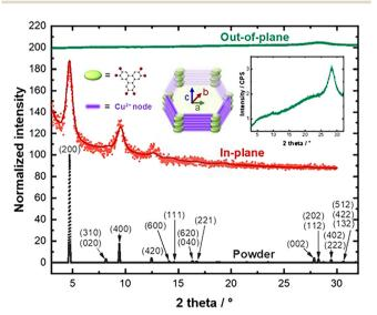
**Fig. 2** Simulated diffractograms of Cu<sub>3</sub>(HHTP)<sub>2</sub> (black); in-plane (red) and out-of-plane (green) XRD measurements.
