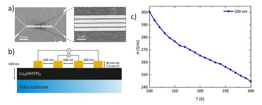
Fig. 4 (a) Scanning electron microscopy image of a contacted for Cu<sub>3</sub>(HHTP<sub>2</sub>) SURMOF. (b) Schematic of experimental setup used for charge transport measurements (c) experimental electrical conductivities ( $\sigma$ ) measured using a 4-point method for Cu<sub>3</sub>HHTP<sub>2</sub> SURMOFs with a thickness of 650 nm. The distance between the contacts amounts to 100 nm
