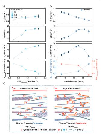
Fig. 5 Thermal Properties of BN/PVA-DX Composite Films. (a) Comparison of heat capacity  $(C_{\rm p})$ , thermal diffusivity  $(\alpha)$ , thermal conductivity  $(\kappa_{\rm c})$ , and  $R_{\rm Kapitza}$  of BN/PVA-DX with varying interfacial HBDs. (b) Comparison of  $C_{\rm p}$ ,  $\alpha$ ,  $\kappa_{\rm c}$ , and  $R_{\rm Kapitza}$  of BN/PVA-D24 composite films with increasing BNNS contents. (c) Schematic diagram depicting phonon transport under low and high interfacial HBD.
