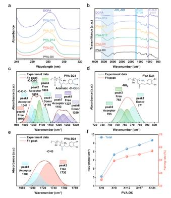
Fig. 2 Characterization, and hydrogen bonding analysis of PVA-DX matrices. (a) Ultraviolet-visible (UV-vis) absorbance spectra of different PVA-D. (b) Fourier-transform infrared (FTIR) spectra of various PVA-D. ATR-FTIR deconvolution of (c) the -C-O(H) region, (d) the  $-NH_2$  region, and (e) the -C=O region in PVA-D24. (f) The hydrogen bond density (HBD) in different PVA-DX matrices.
