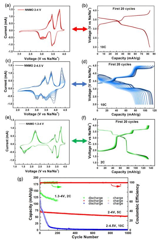
Fig. 1 (a) Cyclic voltammograms (CVs) of NNMO cycled in the 2-4 V window, (b) the corresponding galvanostatic cycling at 10C. (c) CVs of NNMO cycled at a higher voltage range of 2-4.5 V, (d) the corresponding galvanostatic cycling at 10C. (e) CVs of NNMO cycled in the region 1.3-4 V, (f) the corresponding galvanostatic cycling at 2C, and (g) long-term stability of NNMO cycled at different voltage ranges.
