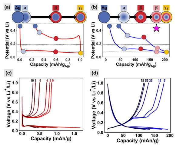
Fig. 5 Voltage profiles and the associated phase transformation in (a) and (c) bulk Aq and (b) and (d) nanoporous Aq anodes. The appearance of the nonequilibrium β solid solution phase in the nanoporous Ag is labelled with the pink star. Reproduced with permission from the American Chemical Society.44
