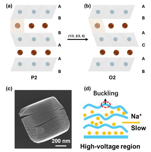
Fig. 2 Chemical structures of (a) P2 and (b) O2 phases of Na<sub>x</sub>[Ni<sub>1/3</sub>Mn<sub>2/3</sub>|O<sub>2</sub>. (c) SEM image of P2-NNMO particles, and (d) schematic illustration of the layered structure after cycling at high voltage showing the formation of cracks and crystal-plane buckling. (c) and (d) Were reproduced with permission from Elsevier.<sup>5</sup>
