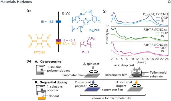
Fig. 1 (a) Molecular structure of P3HT,  $P(q_42T-T)$  and  $P(q_42T-T)$ -5.1 eV for P(g<sub>4</sub>2T-T) and P3HT, respectively) and the electron affinity of the dopant (EA = -5.2 eV). 11.36 (b) Schematic for the preparation of doped polythiophene films with A. co-processing or B. sequential doping. Nanometer and micrometer thick films were prepared for the different characterization experiments. (c) Linecuts from out-of-plane (OOP) and in-plane (IN) GIWAXS data of the doped films.
