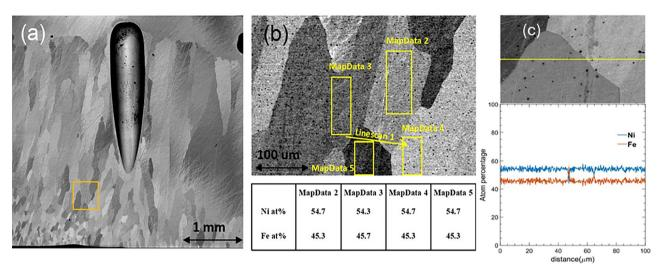
Fig. 6 SEM backscattered electron image on the cross-section of the arc-melted Ni<sub>55</sub>Fe<sub>45</sub> sample (a), the yellow square marked area is the chosen EDS mapping area. This area is enlarged in (b) where the EDS mapping locations on different grains are reported and summarized in the table. (c) EDS line scan across the grains over the line scan 1 shown in (b).
