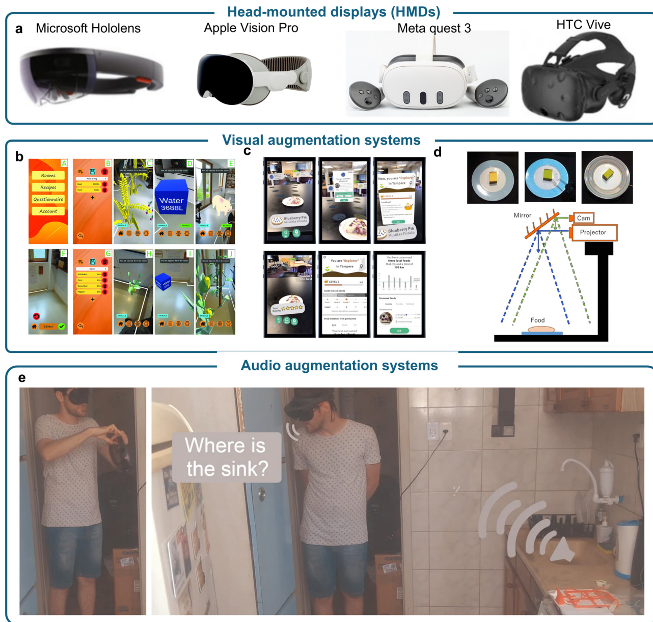
Fig. 5 Strategies for synthesizing images and sounds to simulate and enhance eating experience. (a) Four representative commercially available head-mounted displays, Copyright 2024, 71 Springer Nature Switzerland AG. (b) A handheld augmented reality APP displaying food resources required for preparing a meal, 74 Copyright 2024, IEEE. (c) A mobile augmented reality solution enhancing the dining experience of tourists enjoying a blueberry pie, 75 Copyright 2020, The Author(s). (d) A projection-based augmented reality system modifying the perceived color of real food. 76 (e) The Microsoft HoloLens providing spatial audio guidance to facilitate cooking in low-light or dark environments, 77 Copyright 2021, IFIP International Federation for Information Processing.
