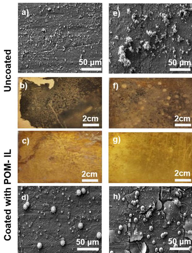
Fig. 7 SEM images (3000 $\times$  magnification) and photographs of uncoated and  $\text{Mo}_8$ -coated brass coupons after incubation in freshwater media: (a)–(d) with microbial communities inhabiting sediment from Schlachtensee, Berlin, for 13 weeks, and (e)–(h) in abiotic freshwater media for 13 weeks.
