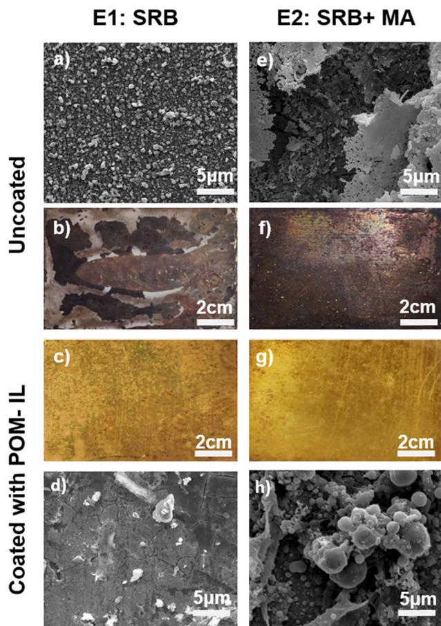
Fig. 6 SEM images (12 000 $\times$  magnification) and photographs of uncoated and  $\text{Mo}_8$ -coated brass coupons after incubation in artificial seawater (ASW) media: (a)–(d) with sulfate-reducing bacteria (SRB) *Desulfovibrio ferrophilus* IS5 for 13 weeks, and (e)–(h) with a 1:1 mixture of methanogenic archaea (MA) *Methanococcus maripaludis* Mic1c10 and SRB *Oleidesulfovibrio alaskensis* 16109 for eight weeks.
