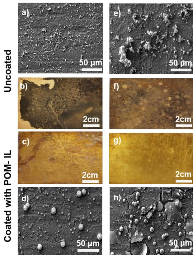
Fig. 7 SEM images (3000 $\times$  magnification) and photographs of uncoated and  $\text{Mo}_6\text{S}_8$ -coated brass coupons after incubation in freshwater media: (a)–(d) with microbial communities inhabiting sediment from Schlachtensee, Berlin, for 13 weeks, and (e)–(h) in abiotic freshwater media for 13 weeks.
