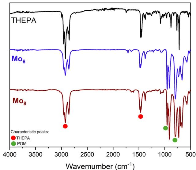
Fig. 2 FT-IR spectra of THEPA,  $\text{Mo}_6$  and  $\text{Mo}_8$ .
