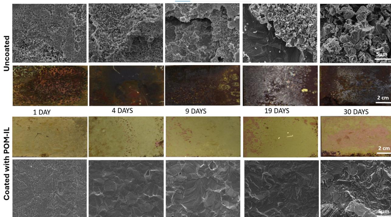
Fig. 4 SEM (10 000 $\times$  magnification) and photographic images of uncoated and POM-IL-coated brass coupons after exposure to 10% of aqueous acetic acid vapour for 1, 4, 9, 19, and 30 days.
