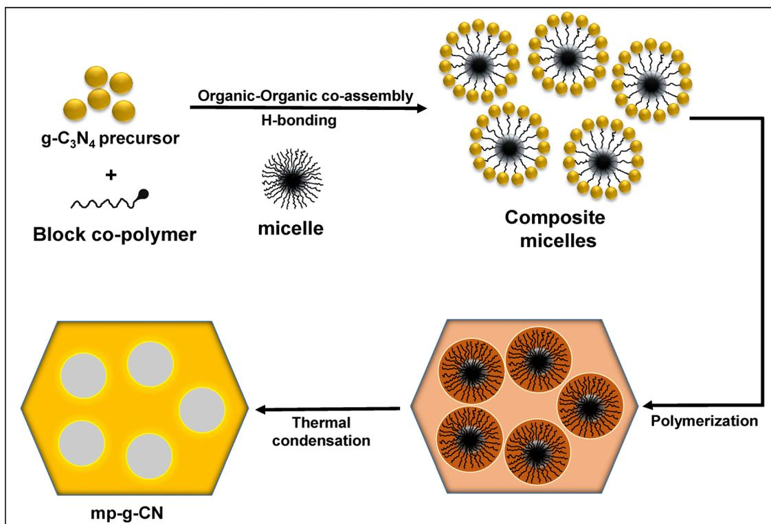
Fig. 9 Stepwise synthesis of a mesoporous g-C<sub>3</sub>N<sub>4</sub>-based photocatalyst using the soft template approach.
