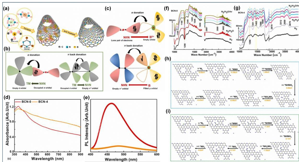
Fig. 52 (a) Schematic depiction of BCN fabrication, schematic depiction of  $\text{N}_2$  adsorption and activation at (b) transition metal and (c) BCN, (d) UV-vis DRS, (e) PL of BCN-0 and BCN-4, *in situ* DRIFT spectra of (f) BCN-0 and (g) BCN-4, DFT analysis of the NRR pathway on (h) BCN-0 and (i) BCN-4. Reproduced with permission.<sup>266</sup> Copyright 2023, Elsevier.
