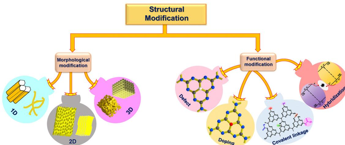
Fig. 17 Schematic illustration of structural modifications in mp-g-CN.
