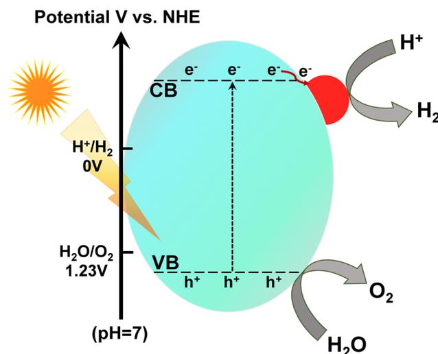
Fig. 32 General mechanism of photocatalytic H<sub>2</sub> evolution.
