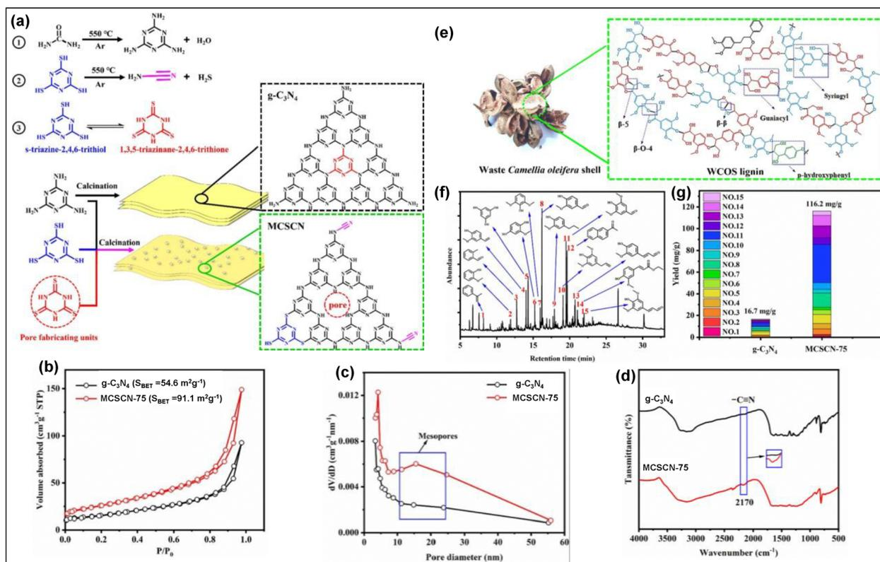
Fig. 59 (a) Schematic depiction of the fabrication of MCSCN, (b)  $\text{N}_2$  adsorption–desorption isotherms, (c) pore-size distribution plot, (d) FT-IR, (e) the proposed structure of waste *Camellia oleifera* shell (WCOS) lignin, (f) GC–MS chromatogram of the reaction mixture, (g) photoactivity of bulk  $g\text{-C}_3\text{N}_4$  and MCSCN-75. Reproduced with permission.<sup>284</sup> Copyright 2022, Elsevier.
