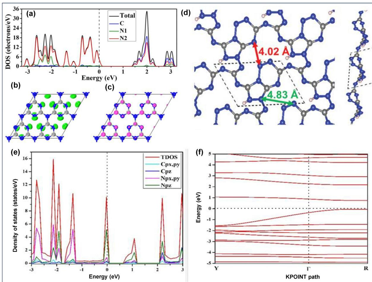
Fig. 30 DFT calculations using the GGA-PBE functional of (a) DOS (the dashed line represents the Fermi energy level), (b) HOMO and (c) LUMO of the g-C<sub>3</sub>N<sub>4</sub> monolayer model. Reproduced with permission.<sup>172</sup> Copyright 2019, Wiley-VCH. (d) Optimized model of the C<sub>3</sub>N<sub>7</sub> monolayer, (e) PDOS and (f) band diagram of C<sub>3</sub>N<sub>7</sub>. Reproduced with permission.<sup>175</sup> Copyright 2019, Wiley-VCH.
