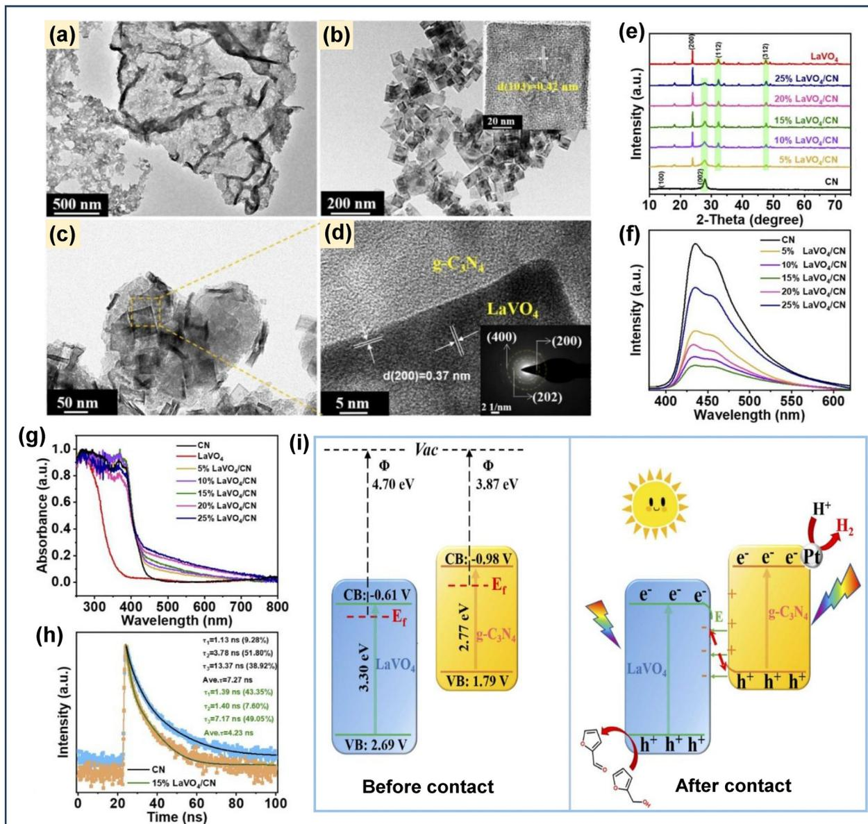
Fig. 63 TEM images of (a) CN, (b) LaVO<sub>4</sub>, (c) LaVO<sub>4</sub>/CN, (d) HRTEM of LaVO<sub>4</sub>/CN, (e) XRD, (f) PL, (g) UV-vis, (h) TRPL, (i) Z-scheme photocatalytic mechanism of LaVO<sub>4</sub>/CN for H<sub>2</sub> and furfural production. Reproduced with permission.<sup>288</sup> Copyright 2022, Elsevier.
