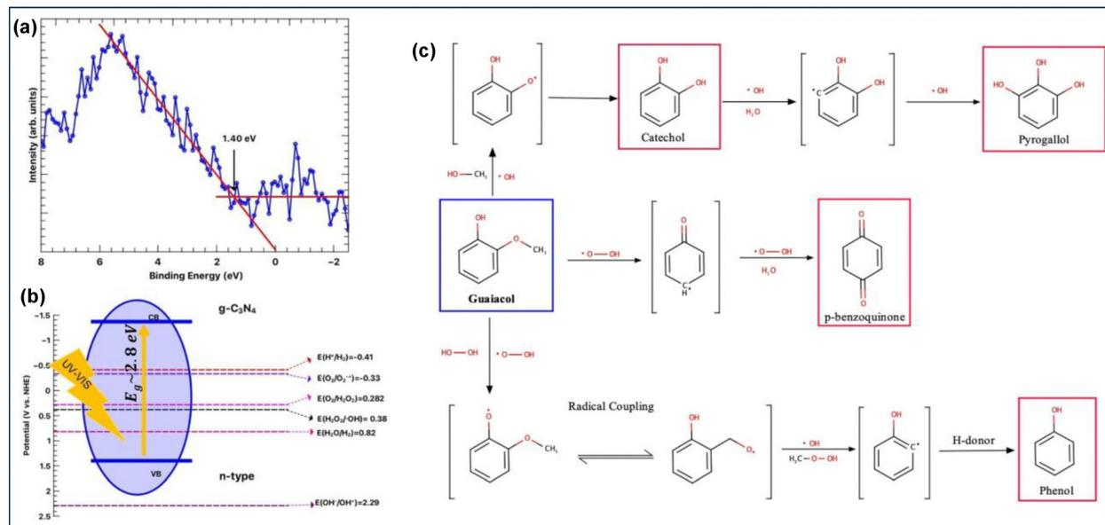
Fig. 60 (a) VB-XPS analysis, (b) band structure and mechanism of light-driven production of ROS, (c) reaction pathway for the photooxidation of guaiacol. Reproduced with permission.<sup>285</sup> Copyright 2021, Elsevier.
