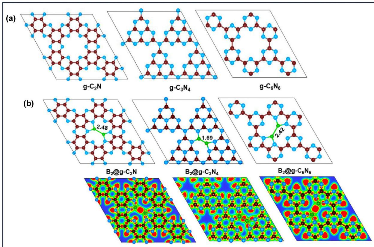
Fig. 31 (a) Calculated optimized models attributed to  $2 \times 2$  monolayers of g-C<sub>2</sub>N, g-C<sub>3</sub>N<sub>4</sub>, and g-C<sub>6</sub>N<sub>6</sub> with a vacuum space of 20 Å along the Z-axis and (b) optimized structure of dual B-doped g-C<sub>2</sub>N, g-C<sub>3</sub>N<sub>4</sub>, and g-C<sub>6</sub>N<sub>6</sub> and related isosurface plot corresponding to the electron localization function. Reproduced with permission.<sup>176</sup> Copyright 2023, American Chemical Society.
