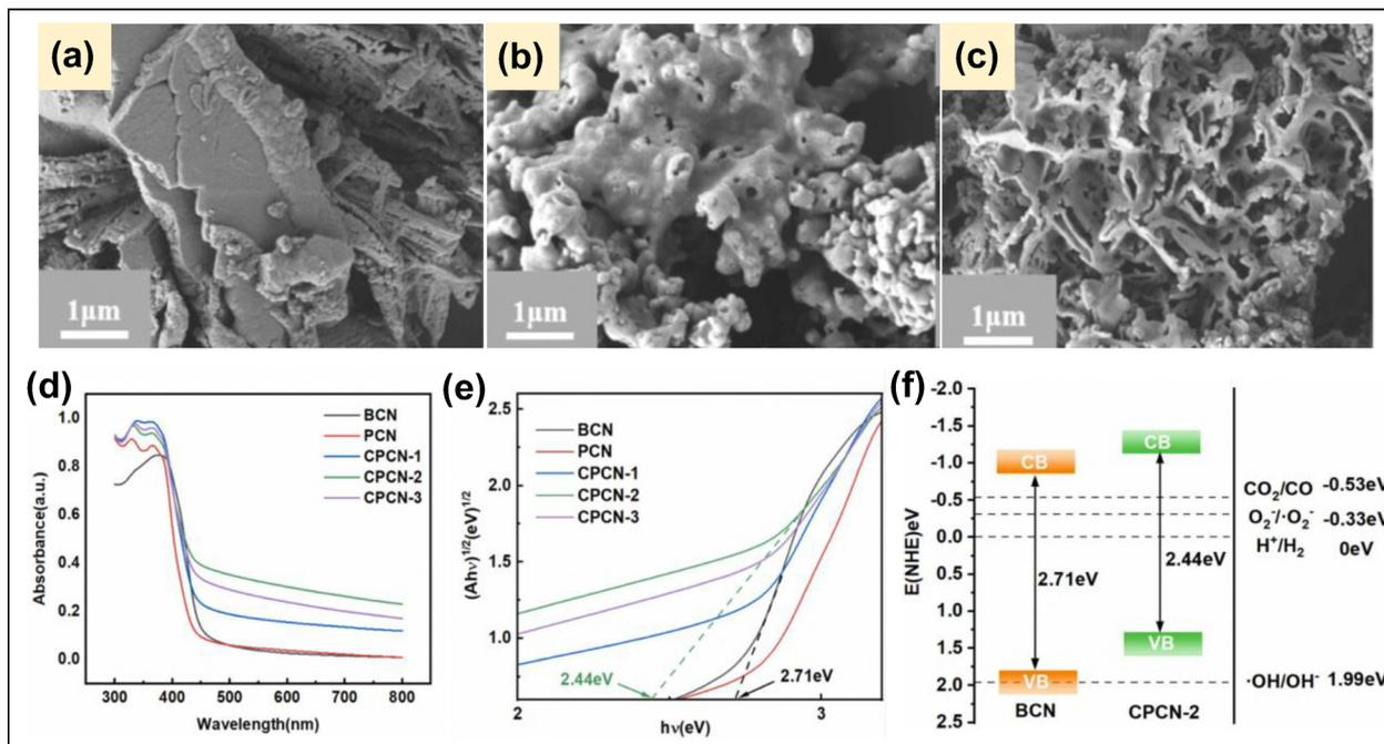
Fig. 41 SEM of (a) BCN, (b) PCN, and (c) CPCN-2, and (d) UV-Vis, (e) band gap energy and (f) band structure analysis of the synthesized materials. Reproduced with permission.<sup>219</sup> Copyright 2024, Elsevier.
