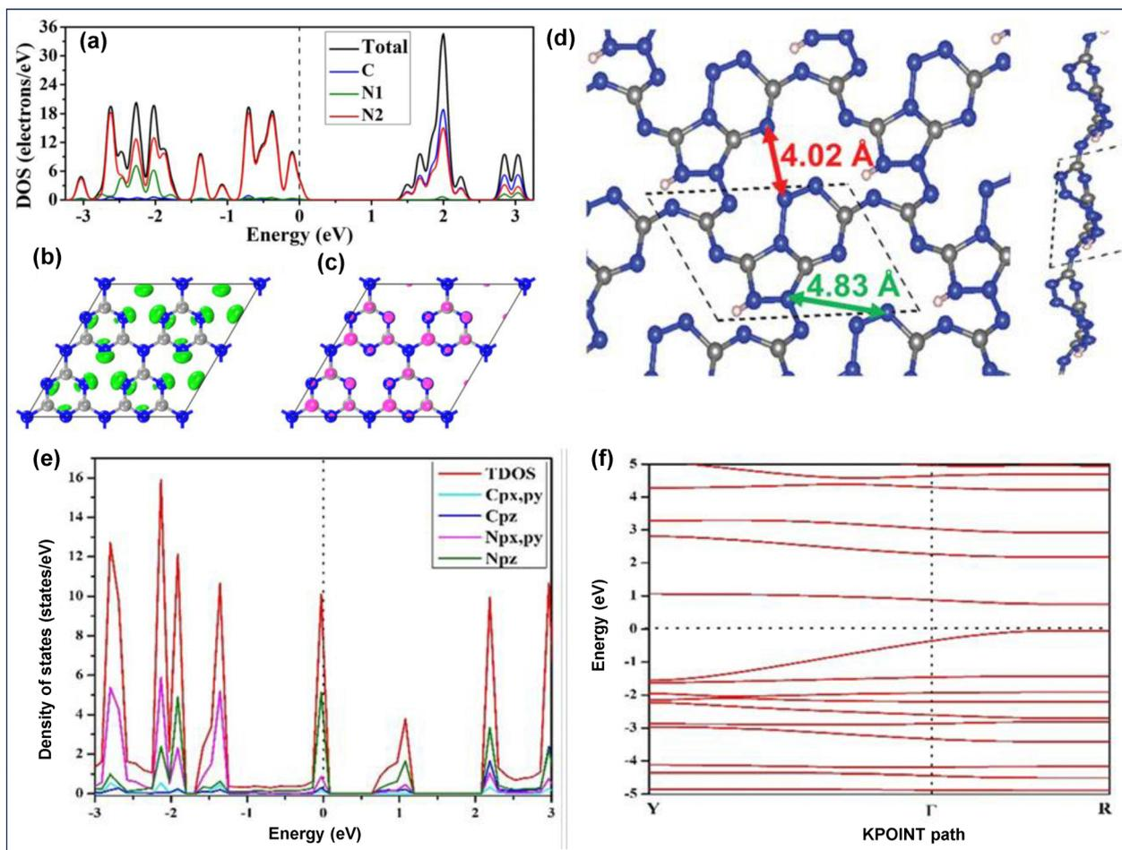
Fig. 30 DFT calculations using the GGA-PBE functional of (a) DOS (the dashed line represents the Fermi energy level), (b) HOMO and (c) LUMO of the  $g$ - $C_3N_4$  monolayer model. Reproduced with permission.<sup>172</sup> Copyright 2019, Wiley-VCH. (d) Optimized model of the  $C_3N_7$  monolayer, (e) PDOS and (f) band diagram of  $C_3N_7$ . Reproduced with permission.<sup>175</sup> Copyright 2019, Wiley-VCH.
