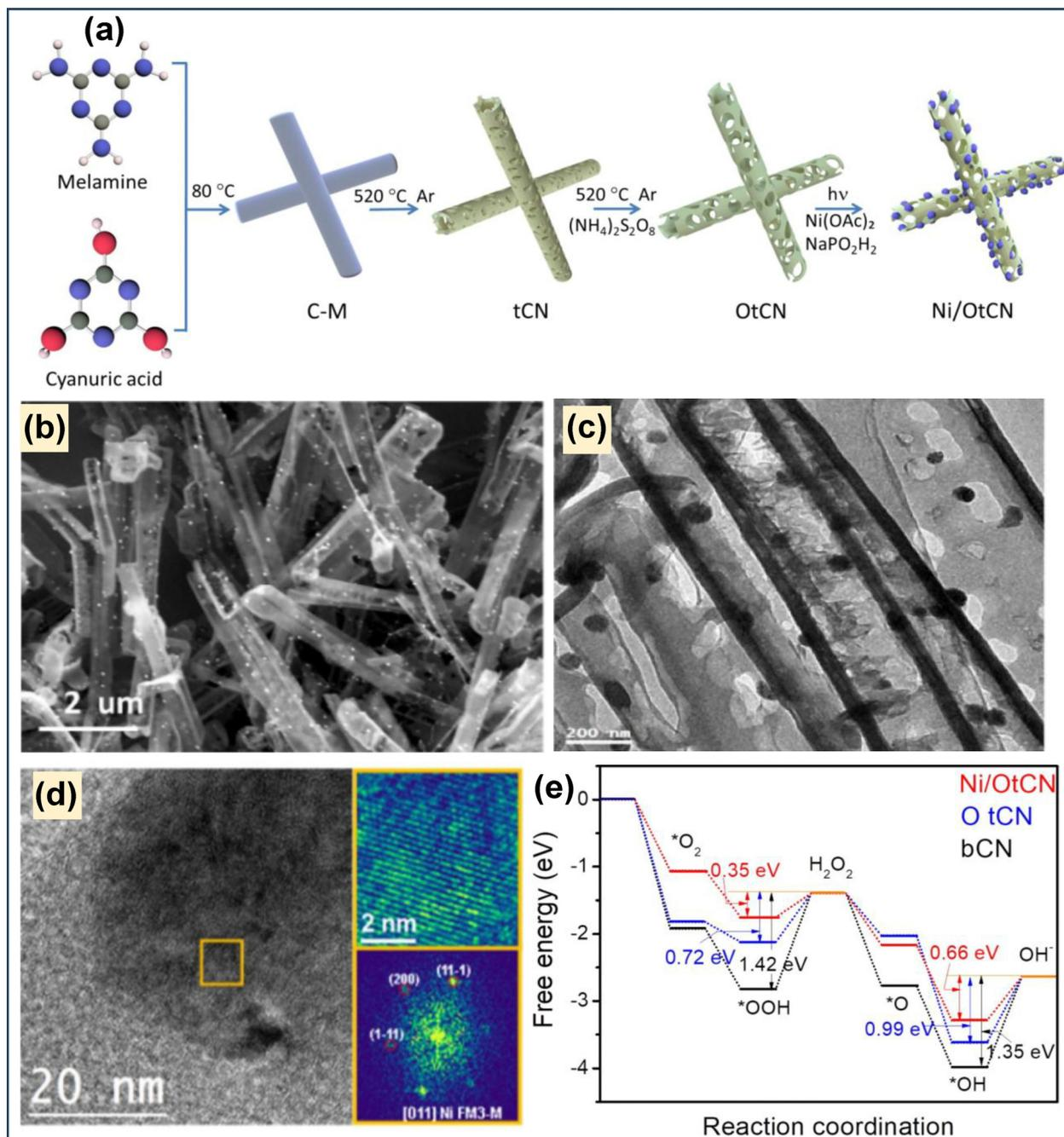
Fig. 49 (a) Diagrammatic representation of the preparation of Ni/OtCN, (b) SEM, (c) TEM, (d) HRTEM image of Ni/OtCN, (e) free energy diagram for ORR. Reproduced with permission.<sup>247</sup> Copyright 2022, Elsevier.
