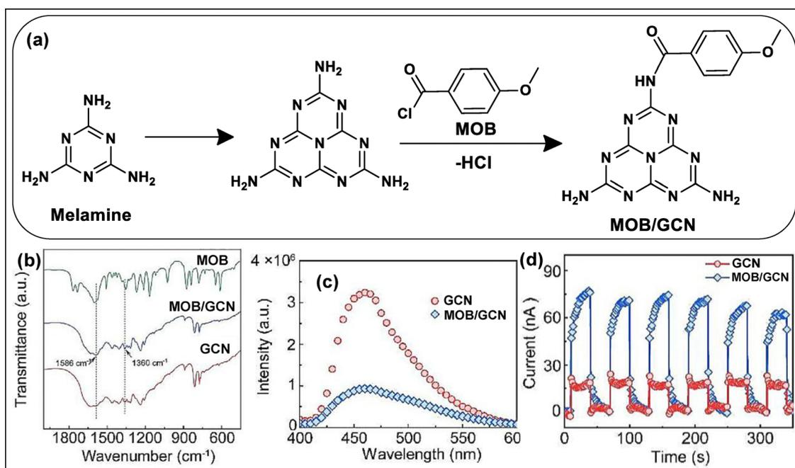
Fig. 26 (a) Diagrammatic representation of MOB/GCN synthesis, (b) FT-IR of MOB, MOB/GCN and GCN, (c) PL, (d) transient photocurrent response of GCN and MOB/GCN. Reproduced with permission.<sup>162</sup> Copyright 2023, Elsevier.
