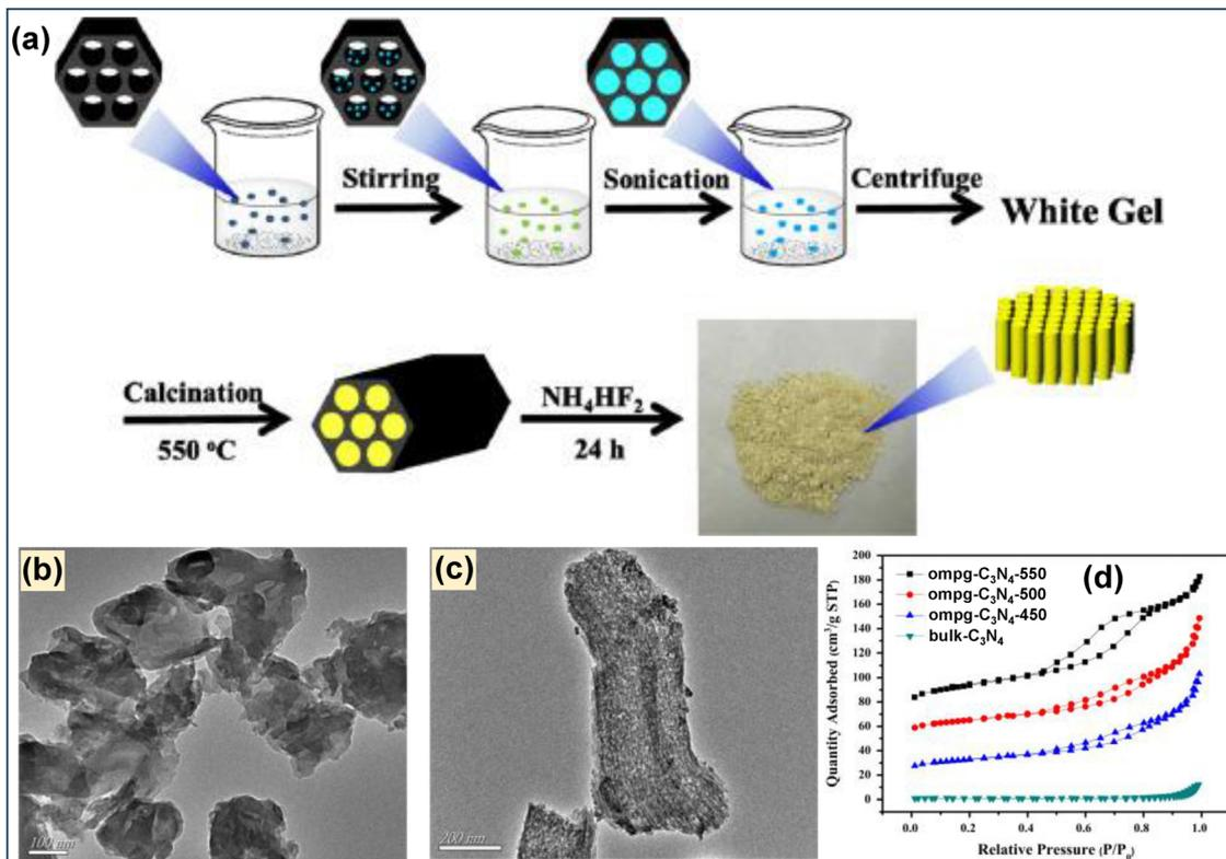
Fig. 6 (a) Diagrammatic sketch of the fabrication of ompg- $C_3N_4$ -550, TEM images of (b) bulk g- $C_3N_4$  and (c) ompg- $C_3N_4$ -550, and (d) BET isotherms of all the CN materials and bulk g- $C_3N_4$ . Reproduced with permission.<sup>79</sup> Copyright 2016, Elsevier (for interpretation of the references to color in this figure legend, the reader is referred to the web version of this article).
