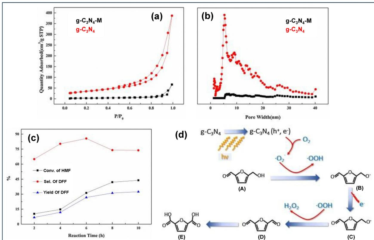
Fig. 57 (a) BET isotherms, (b) pore size distribution plot of the samples, (c) time-dependent photocatalytic activity of  $g\text{-C}_3\text{N}_4\text{-M}$ , (d) mechanism for the photooxidation of HMF to DFF using  $g\text{-C}_3\text{N}_4\text{-M}$ . Reproduced with permission.<sup>282</sup> Copyright 2017, Elsevier.
