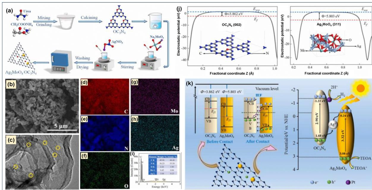
Fig. 39 (a) Schematic depiction of  $\text{Ag}_2\text{MoO}_4/\text{OC}_3\text{N}_4$  synthesis, (b) SEM, (c) TEM, (d)–(h) elemental mapping, (i) EDS profile of  $\text{Ag}_2\text{MoO}_4/\text{OC}_3\text{N}_4$ , (j) optimized work functions of  $\text{OC}_3\text{N}_4$  and  $\text{Ag}_2\text{MoO}_4$ , (k) diagrammatic illustration of the energy level, band bending and photocatalytic  $\text{H}_2$  production mechanism. Reproduced with permission.<sup>201</sup> Copyright 2024, Elsevier.
