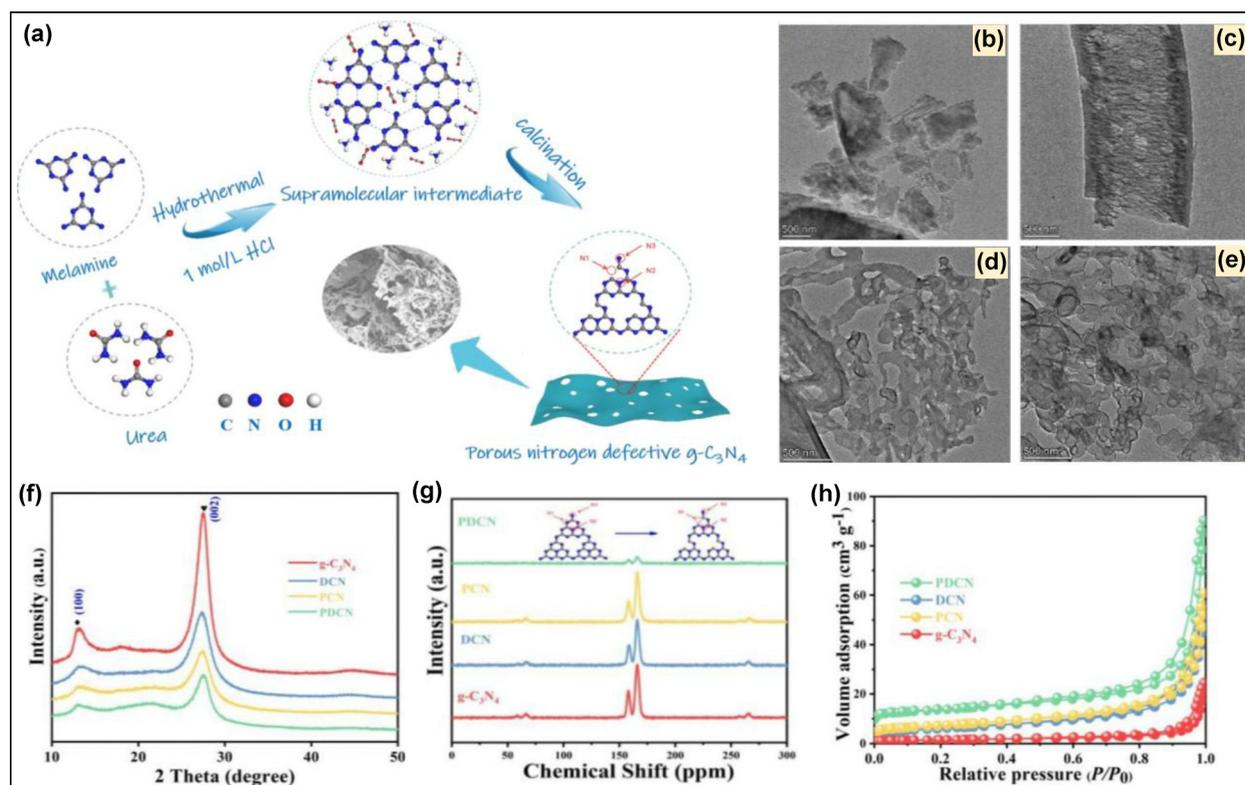
Fig. 21 (a) Fabrication process of PDNC, TEM images of (b)  $g\text{-C}_3\text{N}_4$ , (c) DCN, (d) PCN, and (e) PDCN, (f) XRD, (g) solid-state  $^{13}\text{C}$  NMR, (h) BET isotherms. Reproduced with permission.<sup>155</sup> Copyright 2022, American Chemical Society.
