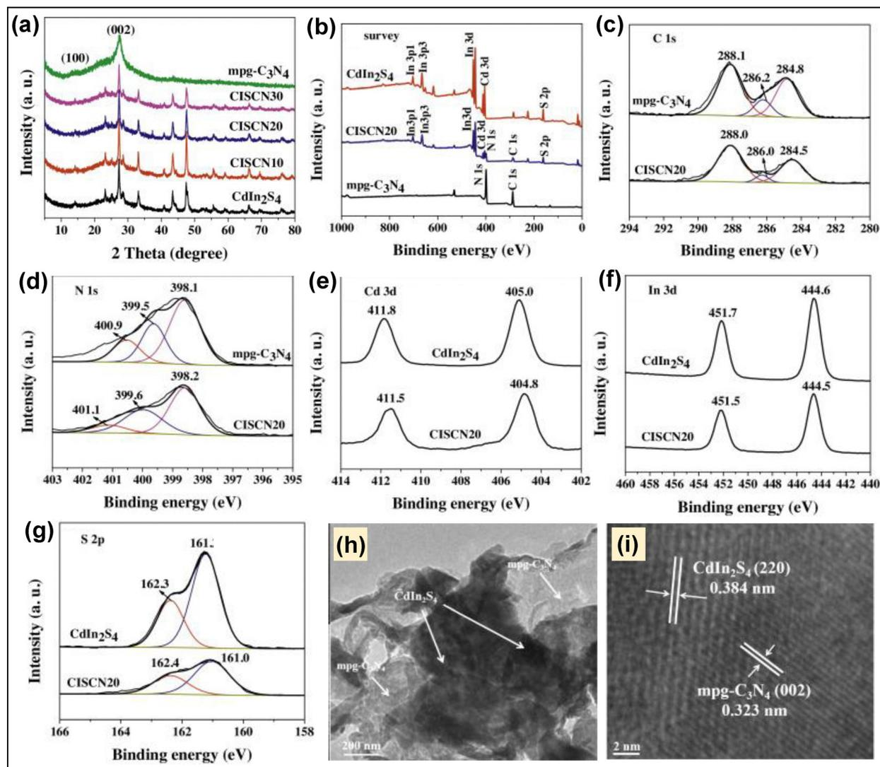
Fig. 28 (a) XRD of all the synthesized samples, (b) XPS survey spectrum of  $\text{CdIn}_2\text{S}_4$ ,  $\text{mpg-C}_3\text{N}_4$ , and CISCN20, (c) C1s and (d) N1s of  $\text{mpg-C}_3\text{N}_4$  and CISCN20, (e) Cd3d, (f) In3d and (g) S2p of  $\text{CdIn}_2\text{S}_4$  and CISCN20, and (h) TEM and (i) HRTEM image of CISCN20. Reproduced with permission.<sup>164</sup> Copyright 2017, Elsevier.
