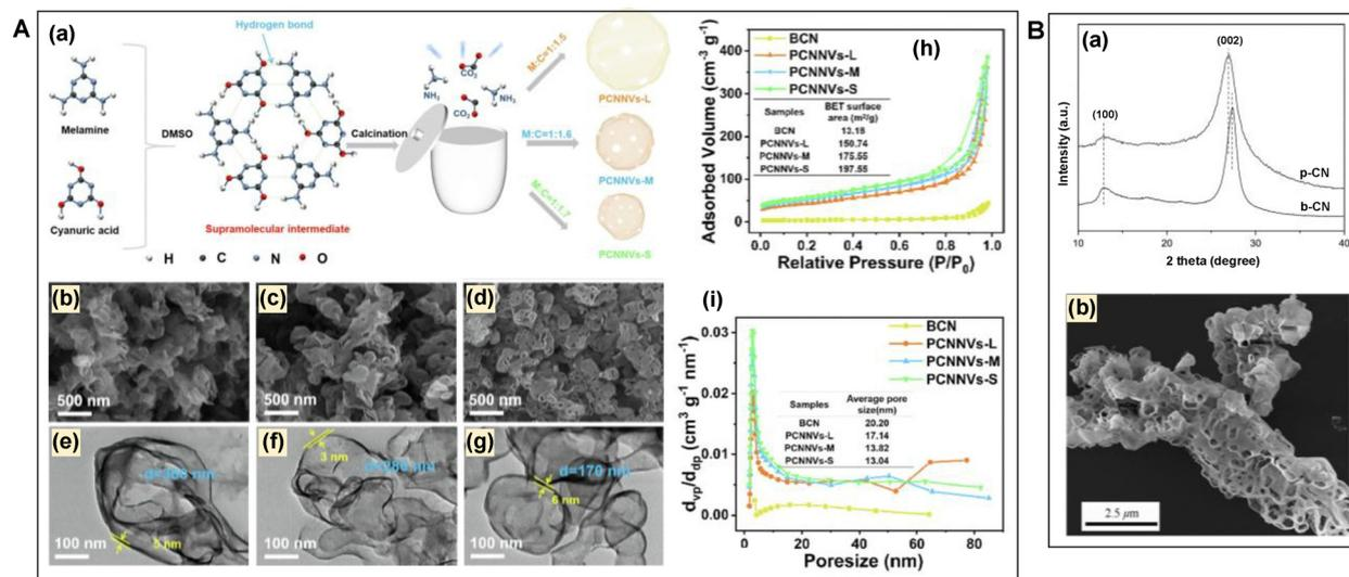
**Fig. 13** (A) (a) Graphical representation of the synthesis of various 3D PCNNV structures, SEM images of (b) PCNNVs-L, (c) PCNNVs-M, (d) PCNNVs-S, TEM image of (e) PCNNVs-L, (f) PCNNVs-M, (g) PCNNVs-S, (h) BET isotherms, (i) pore size distribution of BCN, PCNNVs-L, PCNNVs-M, and PCNNVs-S. Reproduced with permission.<sup>104</sup> Copyright 2022, Elsevier. (B) (a) PXRD of b-CN and p-CN, (b) SEM of p-CN. Reproduced with permission.<sup>105</sup> Copyright 2014, Elsevier.
