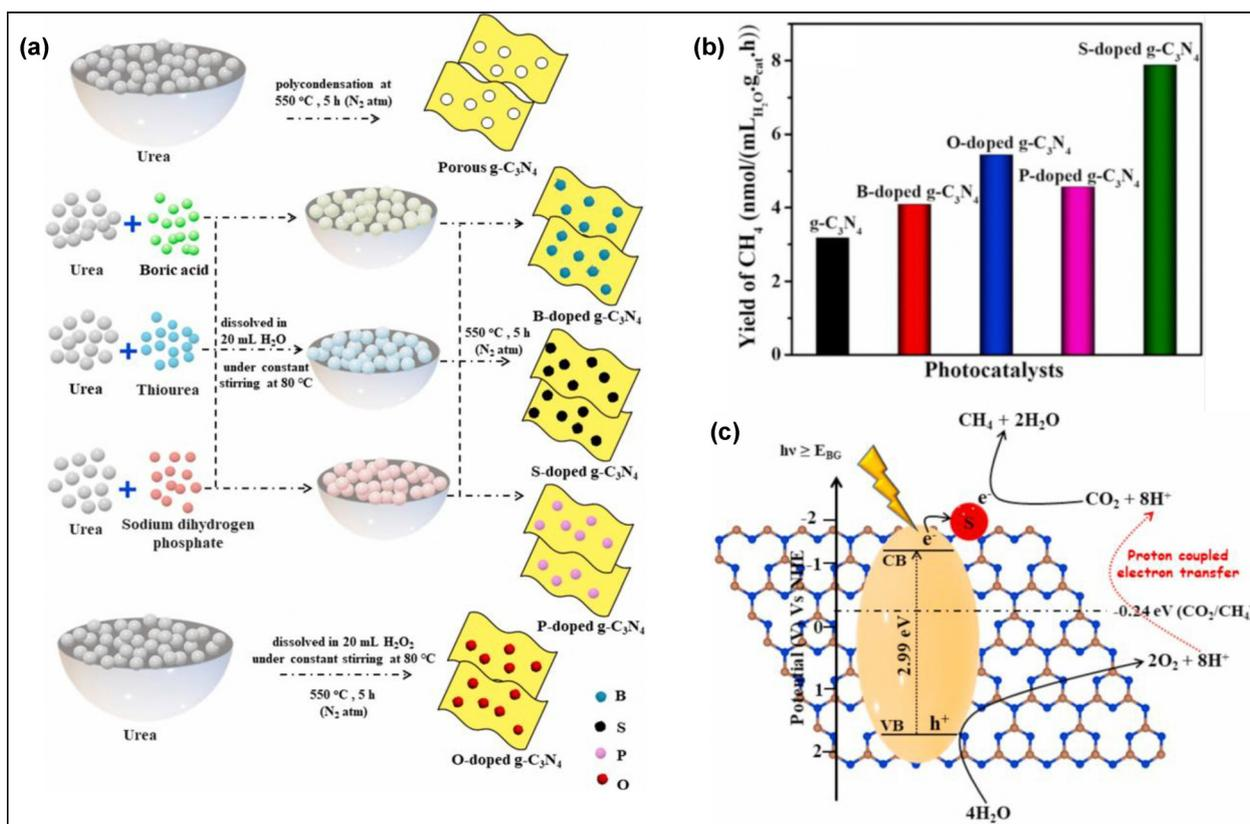
Fig. 43 (a) Diagrammatic representation of the synthesis of mp-g-CN and non-metal (B, O, P, S) doped mp-g-CN, (b) photocatalytic  $\text{CO}_2$  reduction rate of the synthesized samples, (c)  $\text{CH}_4$  production mechanism via photocatalytic  $\text{CO}_2$  reduction. Reproduced with permission.<sup>221</sup> Copyright 2022, Elsevier.
