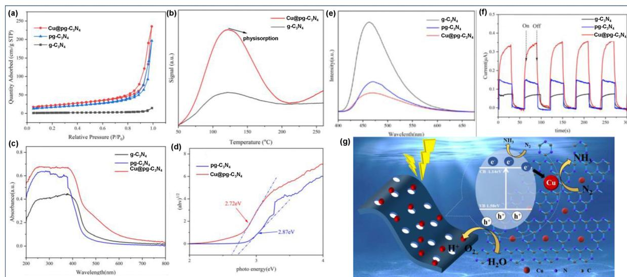
Fig. 54 (a)  $N_2$  adsorption–desorption isotherms, (b)  $N_2$ -TPD profiles, (c) UV-Vis DRS analysis, (d) band gap energies, (e) steady-state PL profile, (f) transient photocurrent analysis of the synthesized photocatalysts, and (g)  $N_2$  photofixation mechanism over  $Cu@pg-C_3N_4$ . Reproduced with permission.<sup>269</sup> Copyright 2023, Wiley-VCH.
