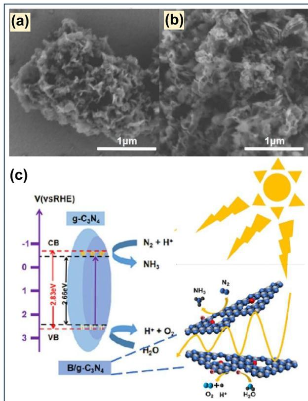
Fig. 51 SEM images of (a)  $\text{g-C}_3\text{N}_4$  and (b) 2 wt% B/g- $\text{C}_3\text{N}_4$ , (c) photocatalytic NRR activity of various synthesized photocatalysts. Reproduced with permission.<sup>265</sup> Copyright 2023, Elsevier.
