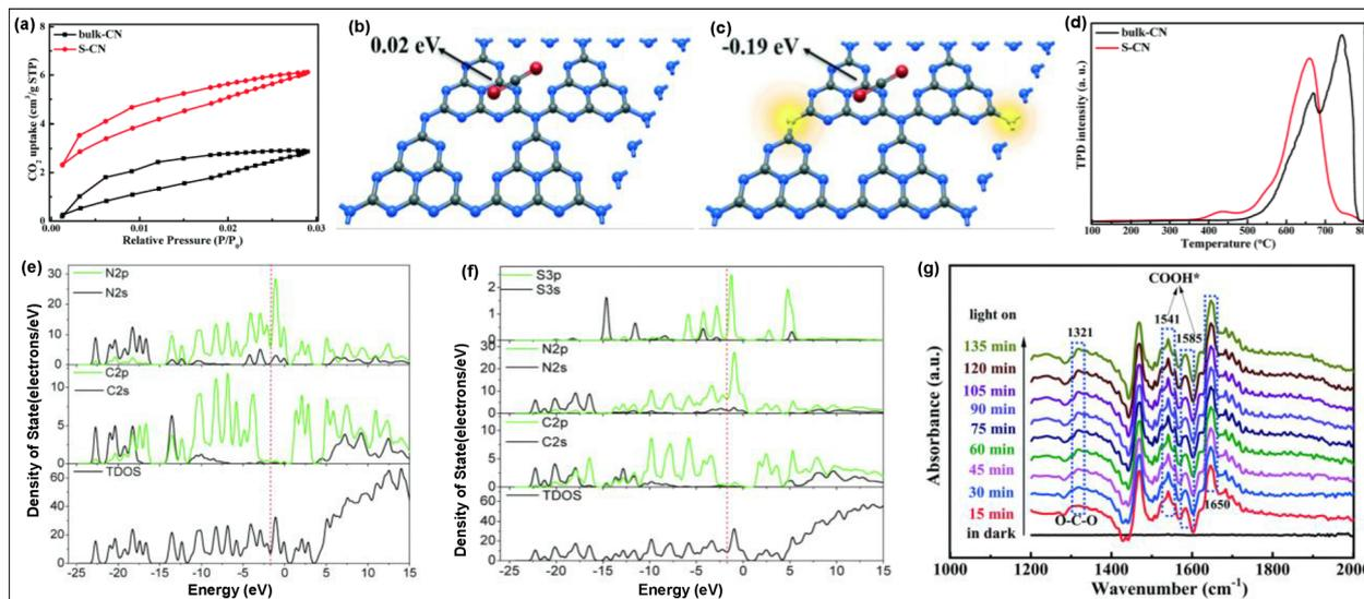
Fig. 42 (a)  $\text{CO}_2$  adsorption isotherms, (b) and (c) DFT study, (d)  $\text{CO}$ -TPD spectra of the samples, (e) and (f) DOS of bulk-CN and S-CN, (g) *in situ* FT-IR spectra. Reproduced with permission.<sup>220</sup> Copyright 2021, The Royal Society of Chemistry.
