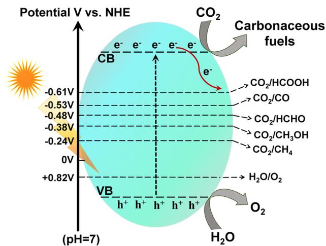
Fig. 40 Schematic depiction of the mechanism of photocatalytic CO<sub>2</sub> reduction.
