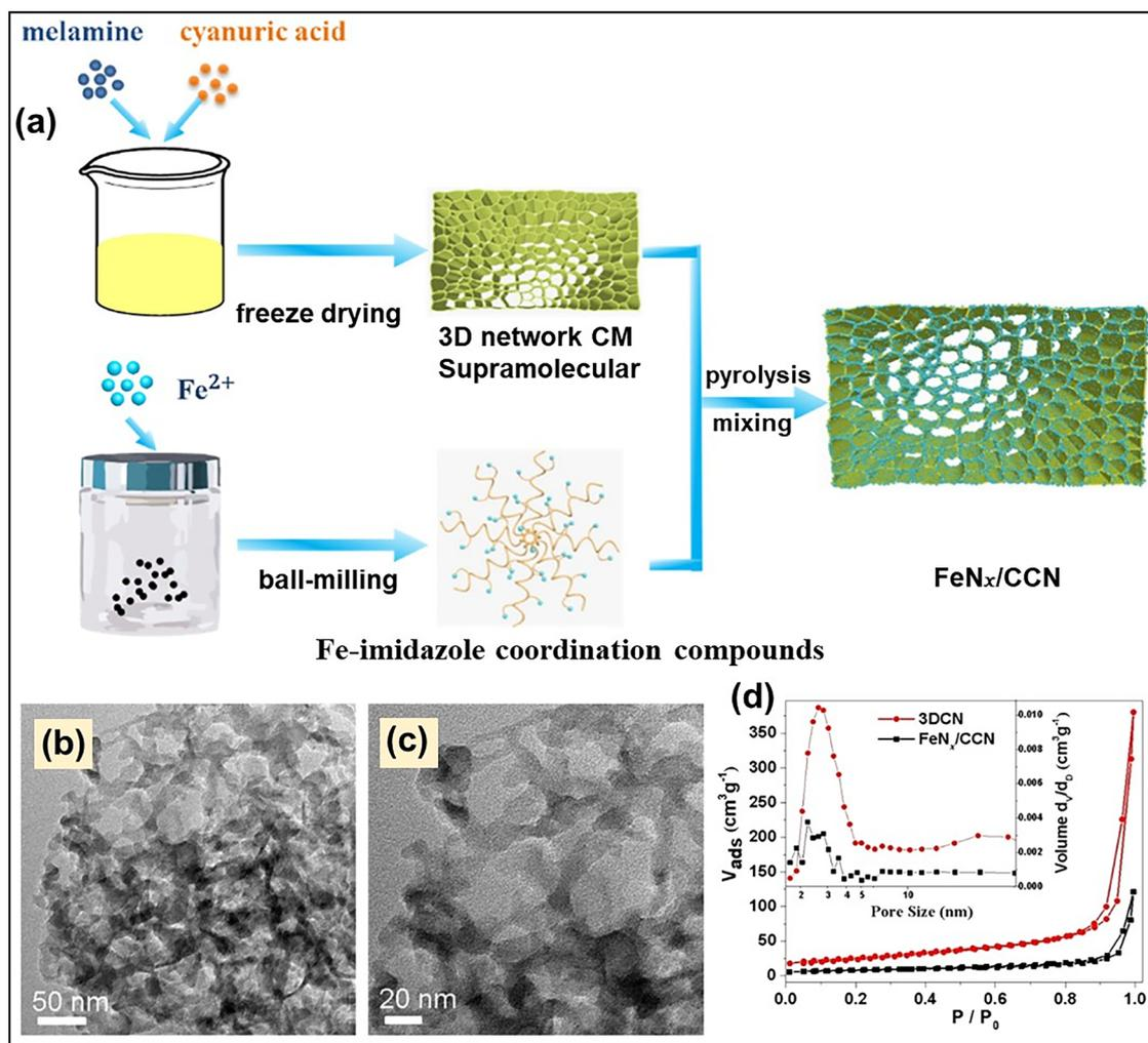
Fig. 14 (a) Schematic illustration of the step-wise synthesis of FeN<sub>x</sub>/CCN, (b) and (c) TEM images of FeN<sub>x</sub>/CCN, (d) N<sub>2</sub> adsorption–desorption isotherm and pore size distribution (inset) of 3DCN and FeN<sub>x</sub>/CCN. Reproduced with permission.<sup>106</sup> Copyright 2023, American Chemical Society.
