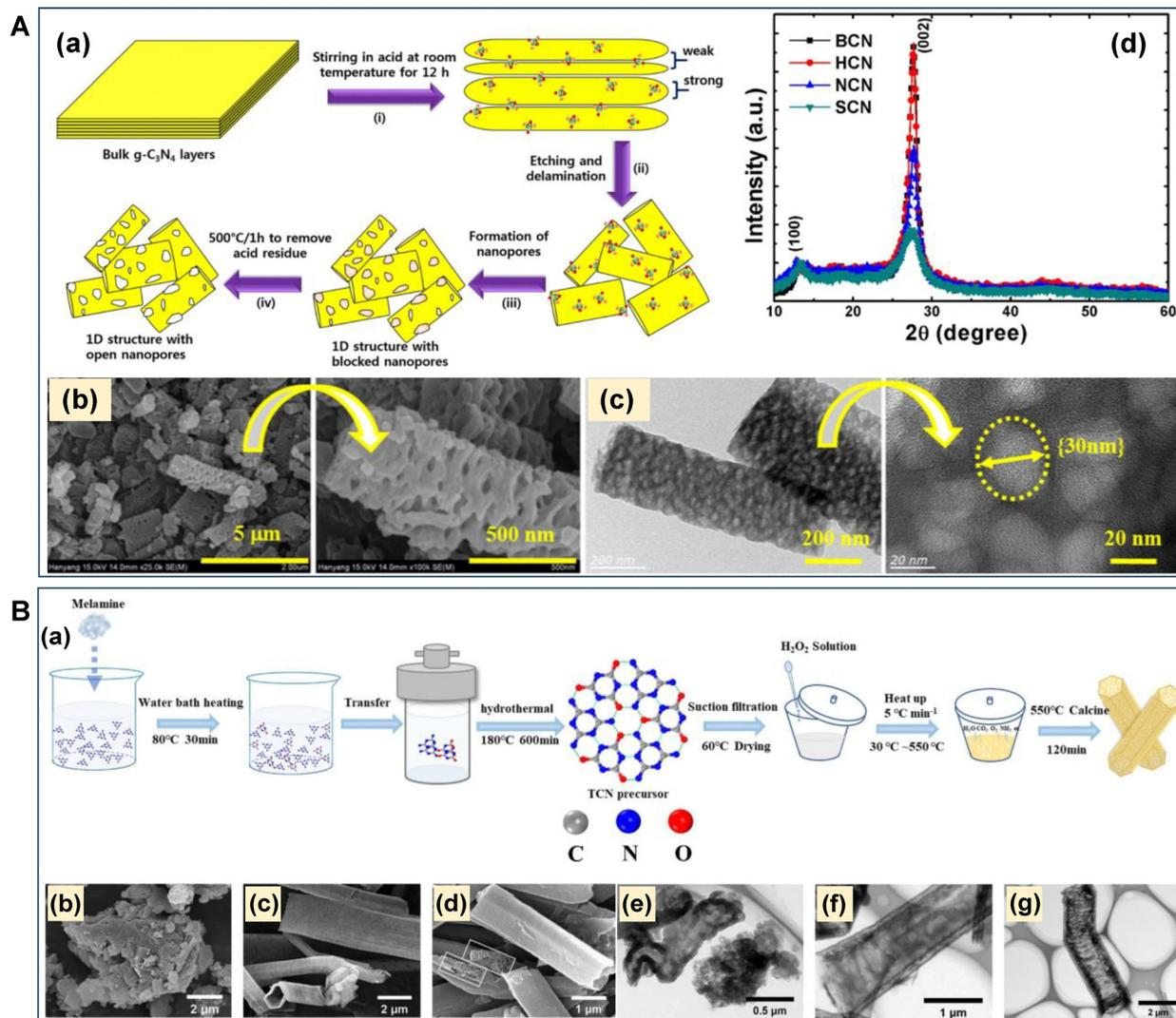
Fig. 18 (A) (a) Schematic depiction of the formation of 1D mp-g-CN nanorods *via* the top-down approach, (b) and (c) SEM and TEM images of SCN, (d) PXRD of all the synthesized materials. Reproduced with permission.<sup>139</sup> Copyright 2016, Nature Communication. (B) (a) Scheme for the step-wise synthesis of AN-TCN, SEM and TEM images of (b) and (e) CN, (c) and (f) TCN and (d) and (g) AN-TCN, respectively. Reproduced with permission.<sup>140</sup> Copyright 2022, Elsevier.
