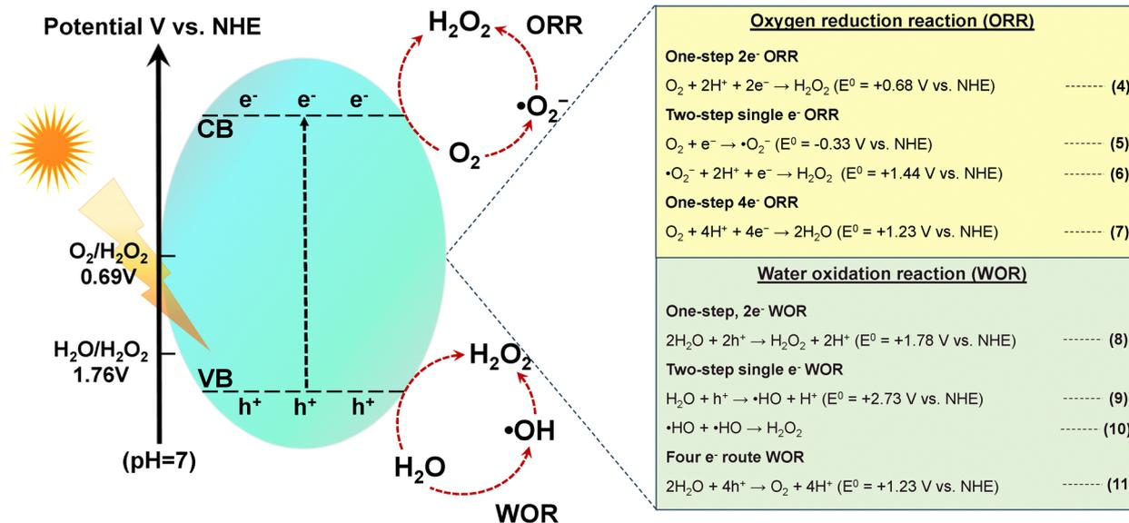
Fig. 45 Schematic overview of the general mechanism of photocatalytic H<sub>2</sub>O<sub>2</sub> production.
