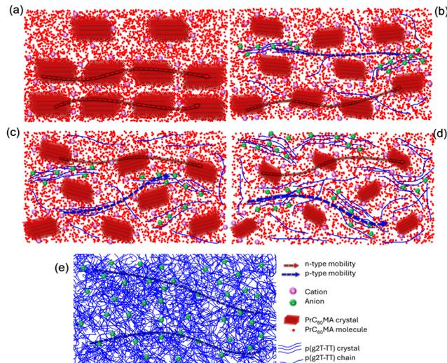
Fig. 6 Microstructure of the p(g2T-TT):PrC<sub>60</sub>MA system, from (a) PrC<sub>60</sub>MA through (b)–(d) 5:95, 10:90, 25:75 to (e) p(g2T-TT). Legend attached in the figure.
