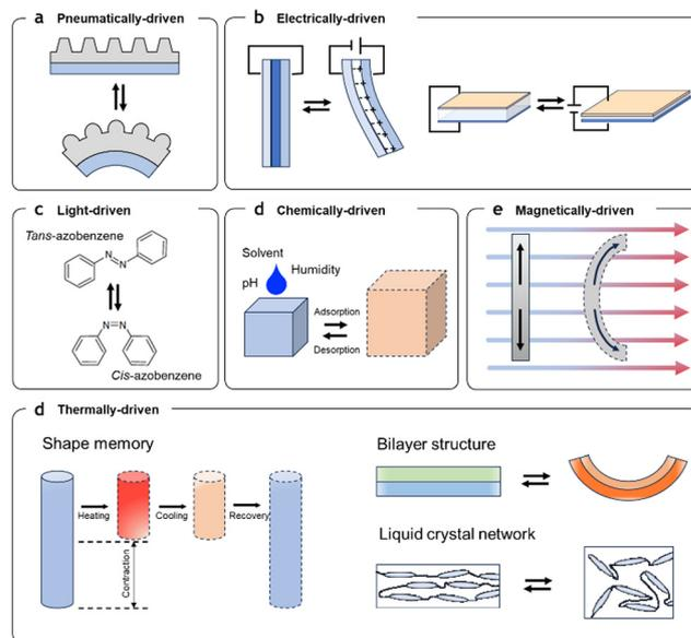
Fig. 2 Schematic illustration of artificial muscles with different actuation mechanisms. Single programming-single actuation mode artificial muscles are designed with pre-memorized states based on the following principles: (a) pneumatically-driven, (b) electrically-driven, (c) light-driven, (d) chemically-driven, (e) magnetically-driven, and (f) thermally-driven mechanisms.
